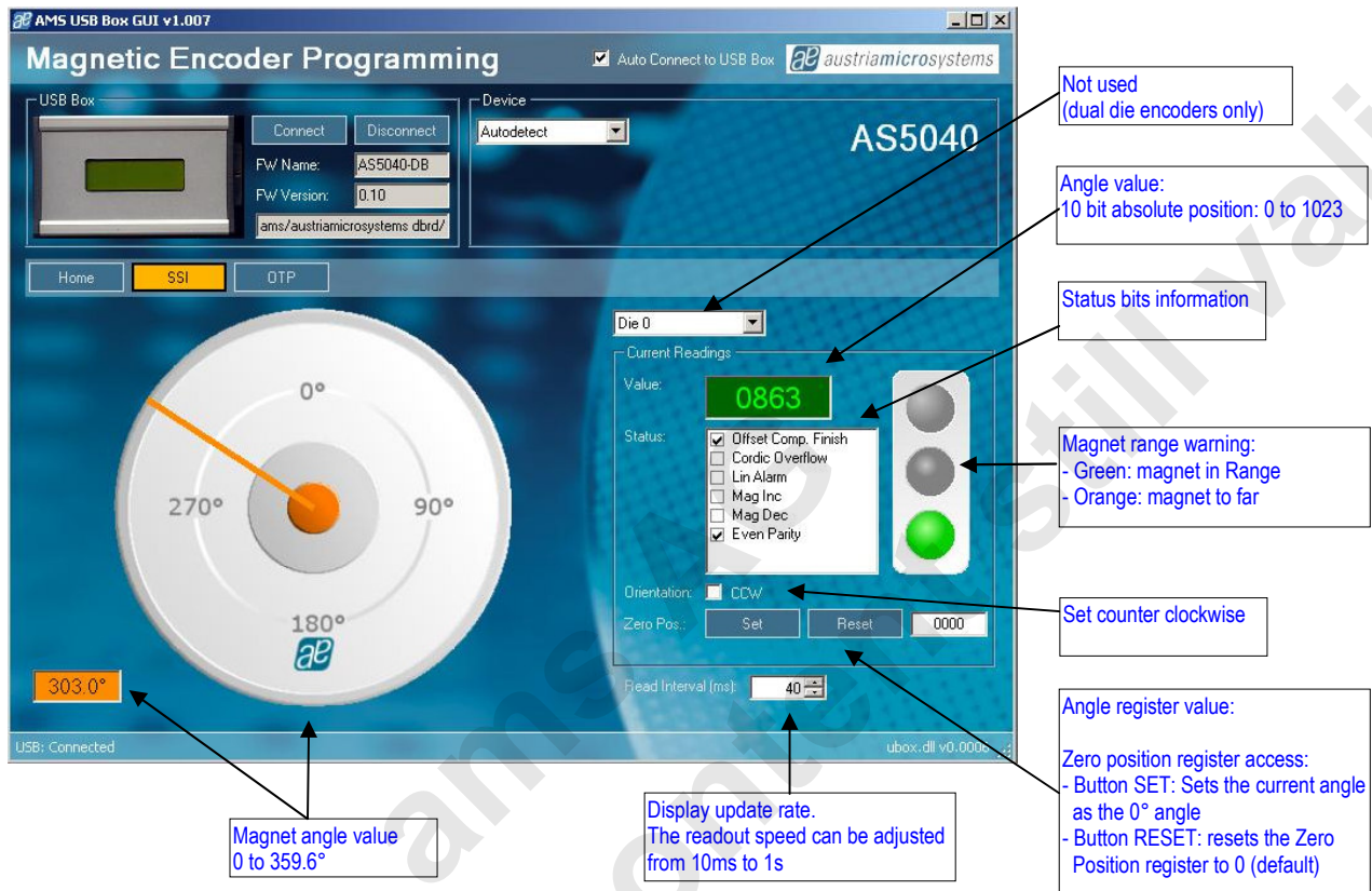
Figure 5: SSI tab, allows access to the AS5X40 registers from the serial bus
