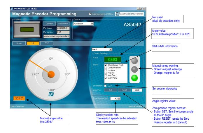
Figure 5: SSI tab, allows access to the AS5X40 registers from the serial bus
