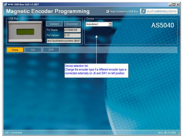
Figure 4: AS5000 GUI detected the AS5040 Demoboard
