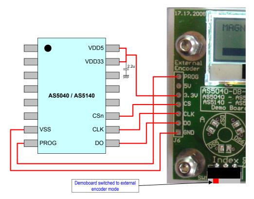
Figure 3: external AS5040/AS5140 connection to the demoboard
