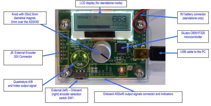
Figure 1: AS5X40 Demoboard hardware with mounted magnet knob
