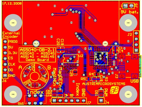
Figure 4: AS5x40 Demoboard PCB Layout
