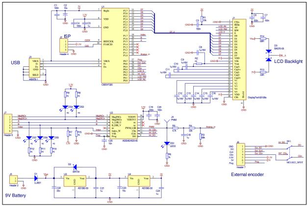
Figure 7: AS5x40 Demoboard schematics
