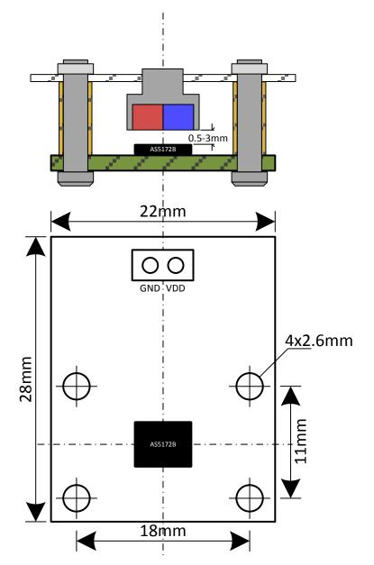
A 8x2.5mm diametric magnet must be placed over or under the AS5172B sensor, and should be centered in the middle of the package with a tolerance of 0.5mm. The airgap between the magnet surface and the package should be maintained in the range 0.5mm to 3mm. The magnet holder must not be ferromagnetic. Materials as brass, copper, aluminum, stainless steel are the best choices to make this part.
