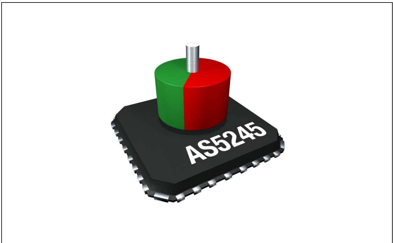
Figure 10: Typical Arrangement of AS5245 and Magnet
