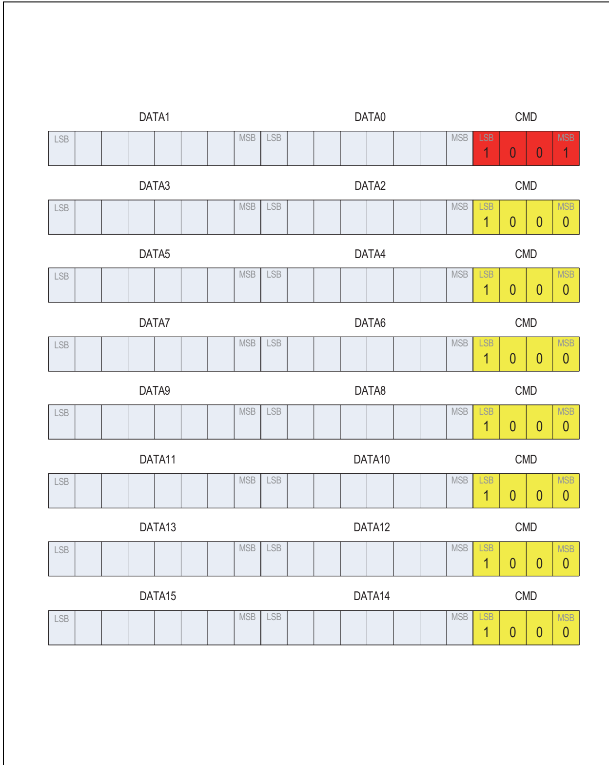
Figure 35: Frame Organization of the WRITE128 Command
