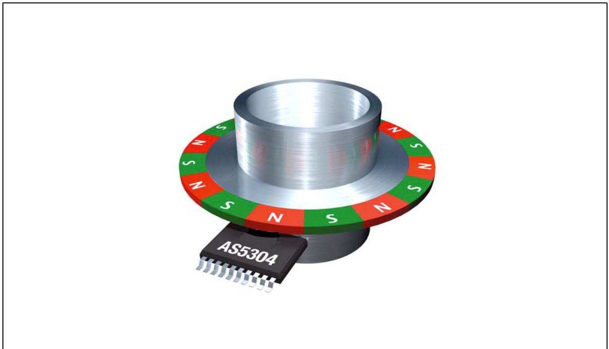
Figure 20: AS5304 (AS5306) with Multi-Pole Ring Magnet
