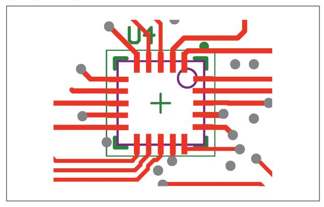
In order to prevent interference, avoid trace routing feedthroughs with exposure directly under the AS7225. An example routing is illustrated in the diagram.
