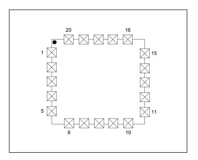
Figure 4: Pin Description of AS7225 (20 pin LGA)
