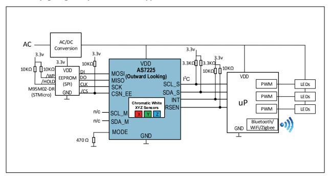
**AS7225 Daylighting and Spectral Presence Application:** AS7225 Outward-looking luminaire integration uses the internal sensor for daylighting and/or spectral presence. CCT-tuning is not supported for outward looking configurations.
