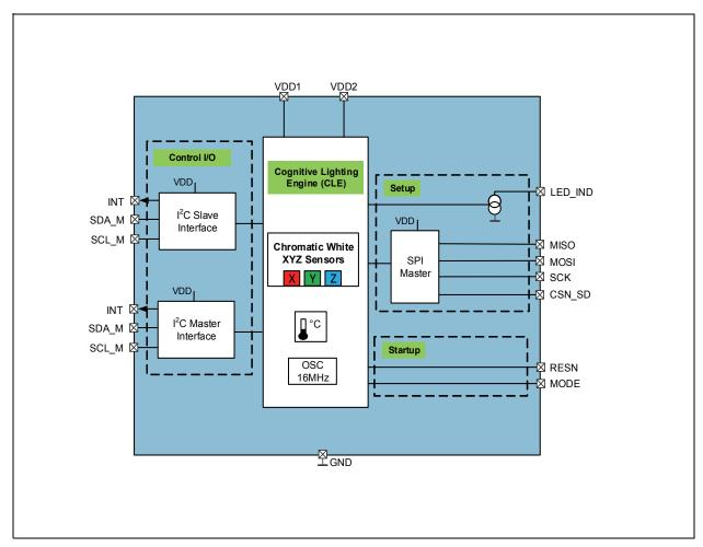
**Block Diagram:** The AS7225 Directs real-time closed loop Chromatic White sensing and PWM tuning to an external host MCU via I<sup>2</sup>C.
