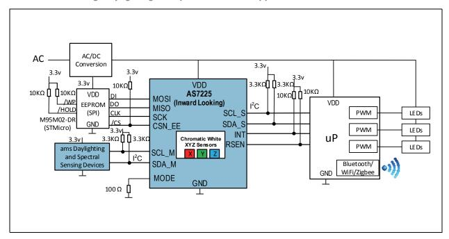
**AS7225 Color Tuning, Daylighting and Spectral Presence Application:** AS7225 <u>Inward-looking</u> luminaire integration requires adding supported sensors via I<sup>2</sup>C for daylighting and/or spectral presence.
