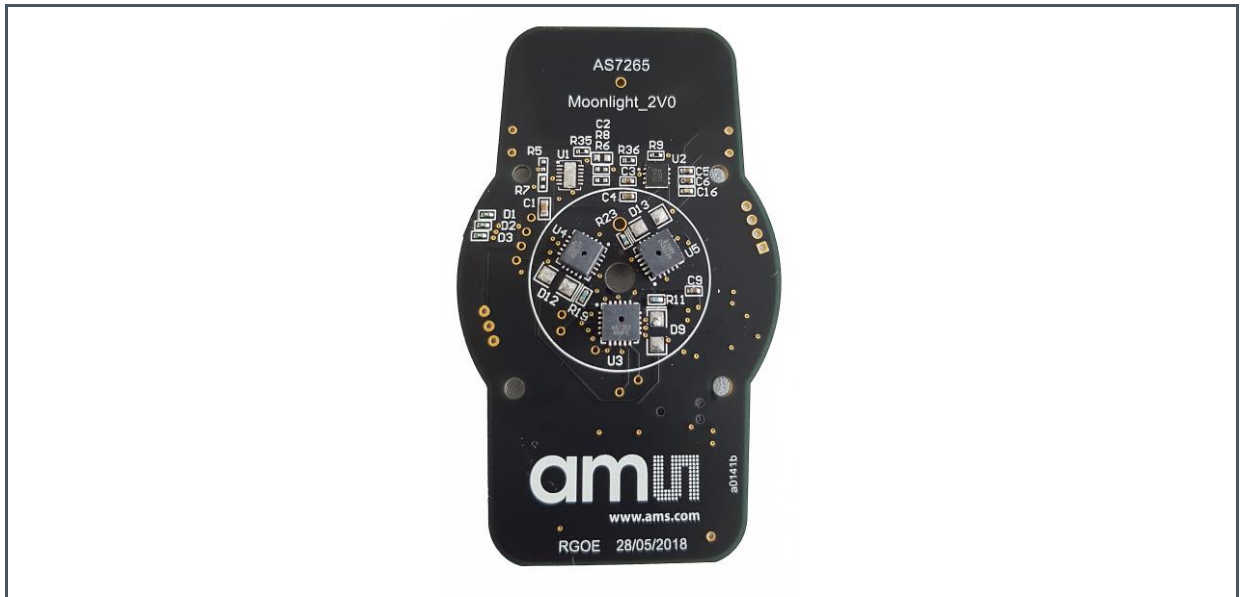
Figure 2: AS7265x Moonlight Multi-Spectral Sensor
