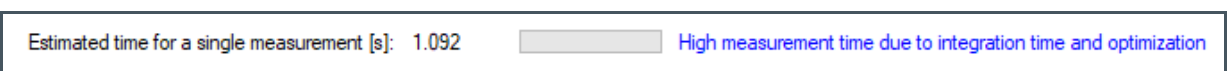
Calculated Measuring Time And Loading Bar In Main Tab If Measuring Time > 1 sec
