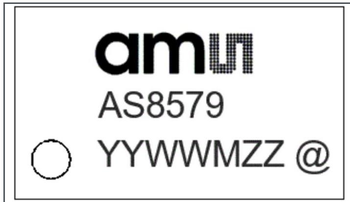
Figure 48: AS8579 Package Marking/Code
