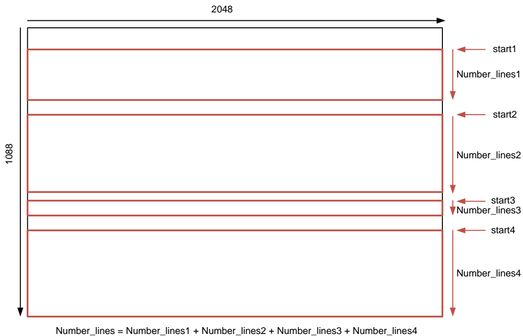
FIGURE 39: EXAMPLE OF 4 MULTIPLE FRAMES READ-OUT
