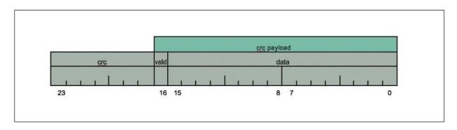
The *checksum* is a cyclic redundancy check over the data and the valid flag; the stored checksum is the result of CRC-7 (polynomial x7+x3+1, see *https://en.wikipedia.org/wiki/Cyclic\_redundancy\_check*) with 0x7F as initial vector (*i.e. with all bits flipped*), see Computing CRC-7 for sample C code.
