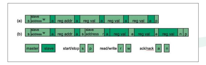
A typical *write* transaction (see Figure 16) therefore has the following format. The master initiates a transaction with a so-called start condition "s". This blocks the bus. Next, the master sends the 7 bits ENS210 *slave address* followed by a 1 bit direction (a 0 indicating write "w"). This byte is acknowledged "a" by the slave. The master continues by sending the 8 bit *register address*, which is acknowledged by the slave.
