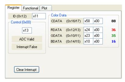
The value of internal registers is displayed on this tab. Register values cannot be set here. To set registers use the Register tab on the input side of the screen.
