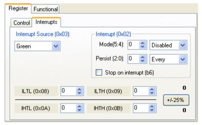
The Interrupt sub-tab allows the user to control the Interrupt pin and the conditions which generate and interrupt, as well as control of the behavior of the interrupt signal itself.
