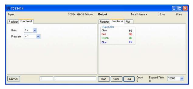
This window has inputs organized on the left, and outputs organized on the right. Values for register variables may be set using multiple techniques. The Functional tab is commonly used to quickly evaluate the device with nominal settings. The Input Register tab allows the register settings to be changed, and the Output Register tab allows registers to be viewed.
