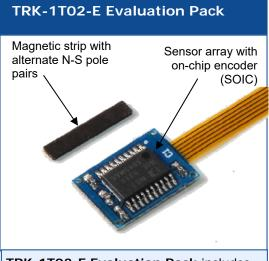
**TRK-1T02-E Evaluation Pack** includes an NSE5310 in a TSSOP 20 package on a board for ease of handling, along with a matching linear magnetic strip. See page 2 for details.
