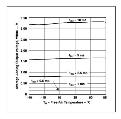
Figure 15: Average Analog Output Voltage, Dark vs. Free-Air Temperature
