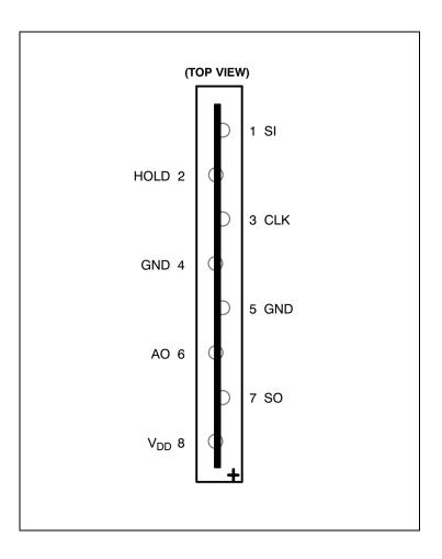
Figure 4: Terminal Functions
