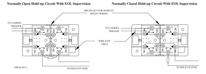
Electrical interlock requires both buttons to be activated simultaneously before alarm will occur. Any single button will activate camera. *Note*: Jumpers required
