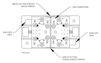
**Converting The HUB-T To Optional Latching Operation** Remove the installed button caps and discard. Replace with alternate latching caps (supplied). Align the cap such that the latching mechanism is directly over the latching ramp in the base. See illustration at right.
