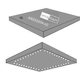
QFN Package mechanical drawing.
