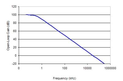
The idealized open loop gain plot is provided for information only. This information is associated with the dpASP in full power mode of operation. The dpASP operational amplifier open loop gain cannot be observed nor used when associated with external connections to the device. Internal reprogrammable routing impedances and switched capacitor circuit architectures using this operational amplifier limit the effective usable bandwidth.
