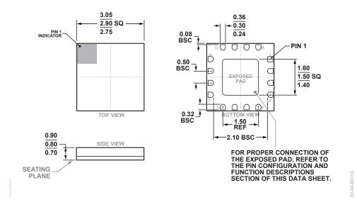
16-Terminal Ceramic Leadless Chip Carrier [LCC] (E-16-1)
