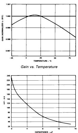
+V<sub>ISO</sub> Ripple vs. Capacitance
