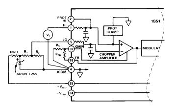
Figure 1. Input Gain Setting and Zero Supression
