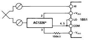
\*PIN NUMBER DEPENDS ON THERMOCOUPLE TYPE SEE AC1226 DATA SHEET FOR DETAILS.
