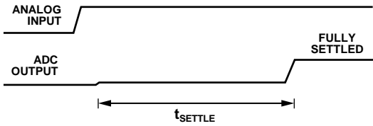
Figure 33. Step Input with Single Cycle Settling
