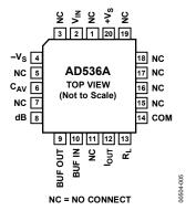
Figure 5. E-20-1 Package Pin Configuration
