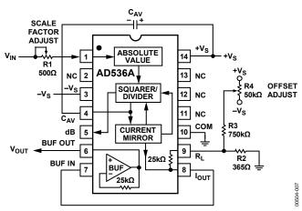
Figure 16. Optional External Gain and Output Offset Trims
