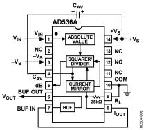
Figure 13. 14-Lead Standard RMS Connection
