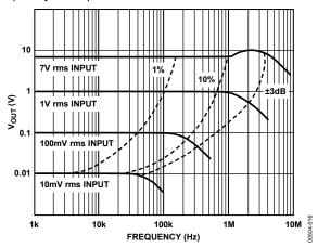
Figure 8. High Frequency Response
