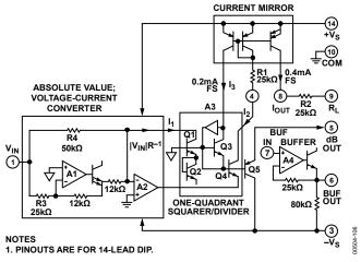
Figure 6. Simplified Schematic
