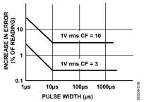
Figure 10. Error vs. Pulse Width Rectangular Pulse
