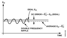
Figure 18. Typical Output Waveform for Sinusoidal Input
