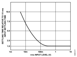
Figure 20. Settling Time vs. Input Level
