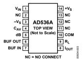
Figure 3. D-14 and Q-14 Packages Pin Configuration
