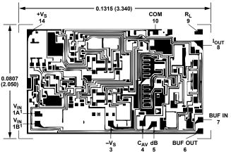
PAD NUMBERS CORRESPOND TO PIN NUMBERS FOR THE TO-100 14-LEAD CERAMIC DIP PACKAGE.
