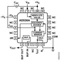
Figure 15. 20-Terminal Standard RMS Connection
