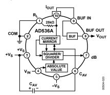
Figure 14. 10-Pin Standard RMS Connection
