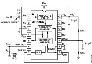
Figure 17. Single-Supply Connection
