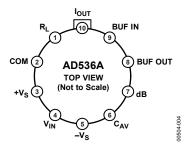
Figure 4. H-10 Package Pin Configuration
