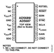
Figure 7. 16-Lead TSSOP Pin Configuration
