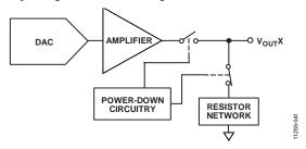
Figure 41. Output Stage During Power-Down
