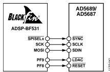
Figure 43. ADSP-BF531 Interface to the AD5689/AD5687
