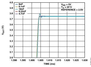
Figure 34. Settling Time vs. Capacitive Load
