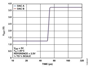
Figure 27. Settling Time, 5 V
