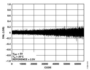
Figure 9. AD5689 Differential Nonlinearity (DNL) vs. Code
