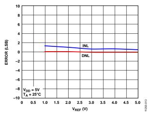
Figure 13. INL Error and DNL Error vs. VRE
