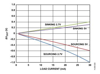
Figure 23. Headroom/Footroom vs. Load Current
