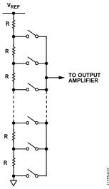
Figure 37. Resistor String Structure
