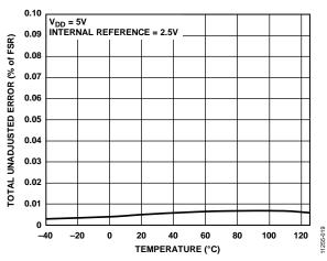
Figure 19. Total Unadjusted Error (TUE) vs. Temperature
