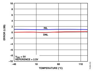
Figure 10. INL Error and DNL Error vs. Temperature
