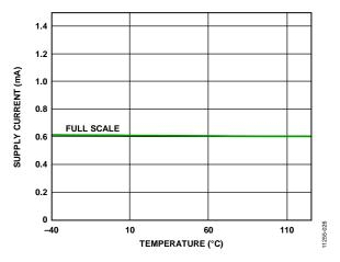
Figure 26. Supply Current vs. Temperature
