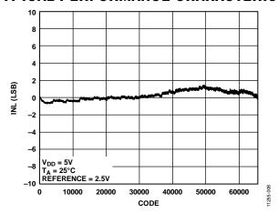
Figure 8. AD5689 Integral Nonlinearity (INL) vs. Code
