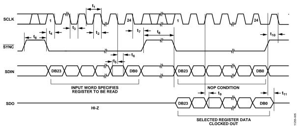
Figure 5. Readback Timing Diagram
