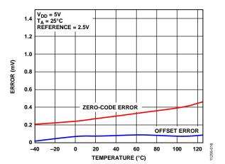
Figure 16. Zero-Code Error and Offset Error vs. Temperature
