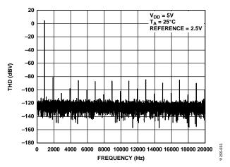
Figure 33. Total Harmonic Distortion at 1 kHz
