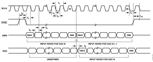
Figure 4. Daisy-Chain Timing Diagram
