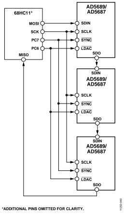
Figure 40. Daisy-Chaining Multiple AD5689/AD5687 Devices
