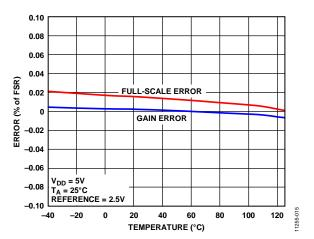
Figure 15. Gain Error and Full-Scale Error vs. Temperature
