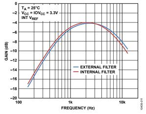
Figure 12. Input Filter Frequency Response
