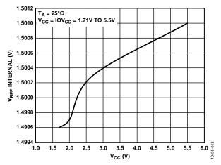
Figure 15. Reference Voltage vs. V<sub>CC</sub>
