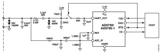
Figure 29. Secondary HART Device
