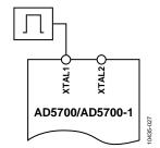
Figure 26. CMOS Clock Connection
