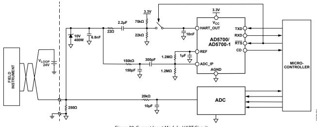
Figure 28. Current Input Module, HART Circuit
