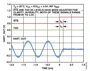
Figure 4. Carrier Stop/Decay Time
