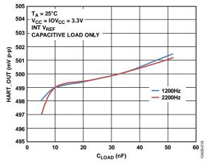
Figure 18. HART\_OUT Voltage vs. CLOAD
