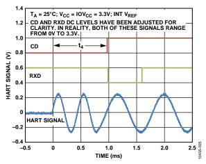
Figure 5. Carrier Detect On Timing
