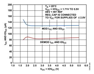
Figure 9. Supply Currents vs. Supply Voltage—Internal Reference
