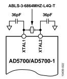
Figure 25. Crystal Oscillator Connection
