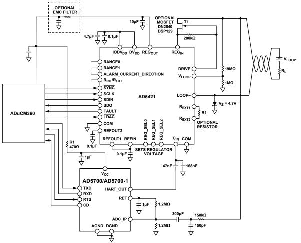
Figure 31. Loop-Powered Transmitter Diagram
