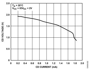
Figure 13. Carrier Detect—Voltage vs. Current, 2 V
