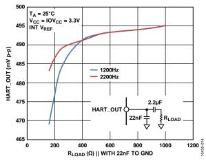
Figure 17. HART\_OUT Voltage vs. R<sub>LOAD</sub>
