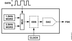
Figure 20. DDS-Based FSK Encoder
