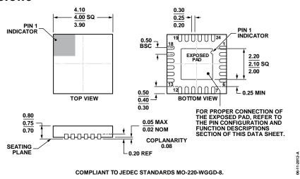
Figure 33. 24-Lead Lead Frame Chip Scale Package [LFCSP\_WQ] 4 mm × 4 mm Body, Very Thin Quad (CP-24-10) Dimensions shown in millimeters
