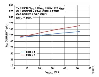
Figure 11. Current in Tx Mode vs. Capacitive Load
