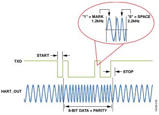
Figure 19. AD5700/AD5700-1 Modulator Waveform
