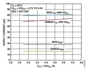
Figure 8. Supply Currents vs. Supply Voltage—External Reference
