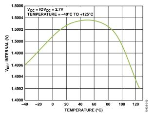
Figure 16. Reference Voltage vs. Temperature
