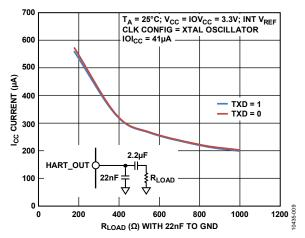
Figure 10. Current in Tx Mode vs. Resistive Load
