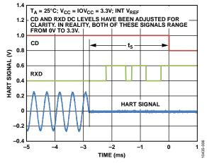
Figure 6. Carrier Detect Off Timing
