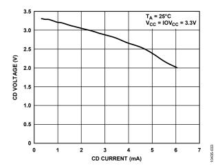
Figure 14. Carrier Detect—Voltage vs. Current, 3.3 V
