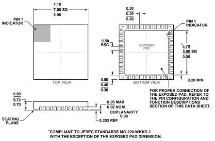
Figure 57. 48-Lead Lead Frame Chip Scale Package [LFCSP] 7 mm × 7 mm Body and 0.75 mm Package Height (CP-48-13) Dimensions shown in millimeters
