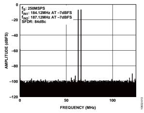
Figure 13. AD6673-250 Two-Tone FFT with  $f_{\rm IN1}$  = 184.12 MHz,  $f_{\rm IN2}$  = 187.12 MHz
