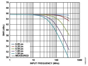
Figure 41. AD6673-250 SNR vs. Input Frequency and Jitter
