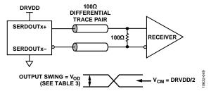
Figure 53. DC-Coupled Digital Output Termination Example
