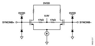
Figure 22. Equivalent SYNCINB± Input Circuit
