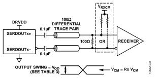
Figure 52. AC-Coupled Digital Output Termination Example
