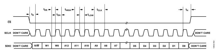
Figure 56. Serial Port Interface Timing Diagram
