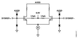
Figure 23. Equivalent SYSREF± Input Circuit
