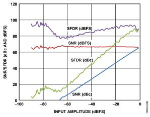
Figure 8. AD6673-250 Single-Tone SNR/SFDR vs. Input Amplitude ( $A_{\rm IN}$ ) with  $f_{\rm IN}=185.1~{\rm MHz}$
