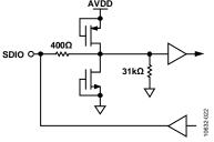
Figure 20. Equivalent SDIO Circuit
