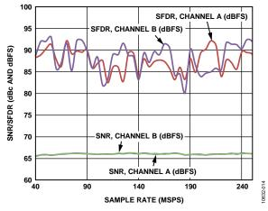
Figure 14. AD6673-250 Single-Tone SNR/SFDR vs. Sample Rate ( $f_{\rm S}$ ) with  $f_{\rm IN}=90.1$  MHz
