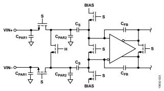
Figure 27. Switched-Capacitor Input
