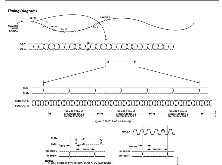
Figure 3. SYSREF± Setup and Hold Timing
