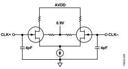
Figure 32. Equivalent Nyquist Clock Input Circuit
