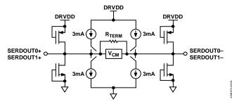
Figure 18. Digital CML Output Circuit
