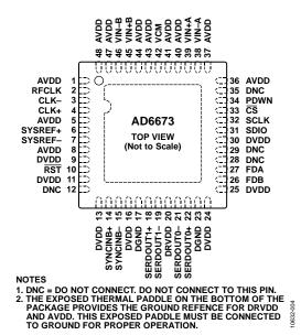
Figure 4. Pin Configuration (Top View)
