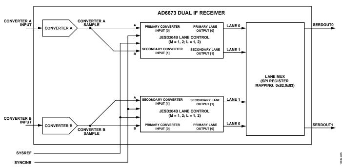
Figure 49. AD6673 Transmit Link Simplified Block Diagram
