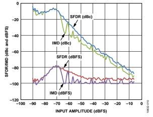
Figure 10. AD6673-250 Two-Tone SFDR/IMD3 vs. Input Amplitude ( $A_{\rm IN}$ ) with  $f_{\rm IN1}=89.12$  MHz,  $f_{\rm IN2}=92.12$  MHz
