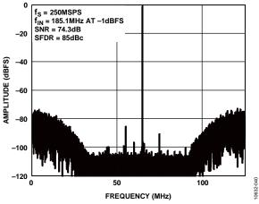
Figure 44. 22% Bandwidth Mode, Tuning Word = 28 (f<sub>5</sub>/4 Tuning)
