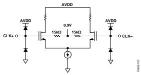
Figure 17. Equivalent Clock Input Circuit
