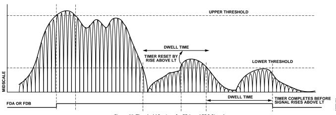
Figure 55. Threshold Settings for FDA and FDB Signals
