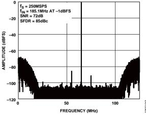
Figure 47. 33% Bandwidth Mode, Tuning Word = 17 ( $f_{\varsigma}/4$  Tuning)
