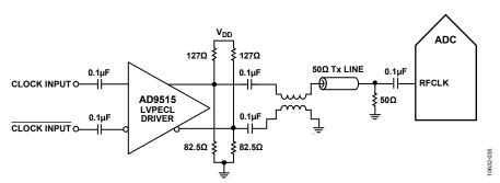
Figure 39. Differential PECL RF Clock Input Circuit
