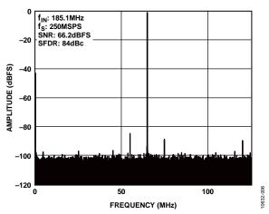
Figure 6. AD6673-250 Single-Tone FFT with  $f_{IN} = 185.1$  MHz
