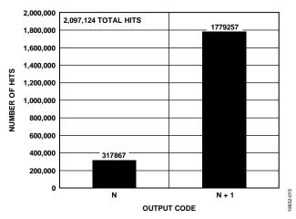
Figure 15. AD6673-250 Grounded Input Histogram
