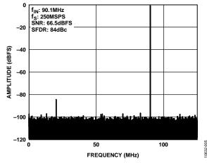
Figure 5. AD6673-250 Single-Tone FFT with  $f_{IN} = 90.1 \text{ MHz}$
