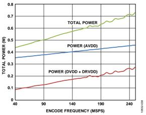
Figure 42. AD6673-250 Power vs. Encode Rate
