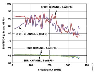
Figure 9. AD6673-250 Single-Tone SNR/SFDR vs. Input Frequency  $(f_{IN})$
