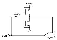
Figure 25. Equivalent VCM Circuit
