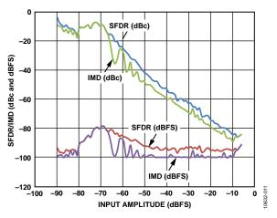
Figure 11. AD6673-250 Two-Tone SFDR/IMD3 vs. Input Amplitude ( $A_{\rm IN}$ ) with  $f_{\rm IN1}=184.12$  MHz,  $f_{\rm IN2}=187.12$  MHz
