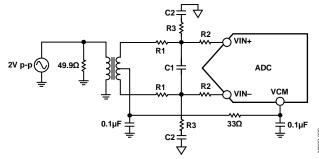
Figure 29. Differential Transformer-Coupled Configuration
