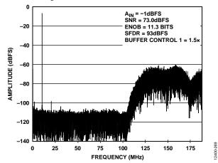
Figure 116. AD6674-750,  $f_{CLOCK} = 750$  MHz,  $f_S = 375$  MSPS,  $f_{IN} = 10.3$  MHz, 28% BW Mode, Tuning Word = 0
