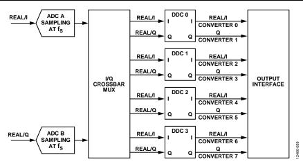
Figure 138. DDCs and Virtual Converter Mapping
