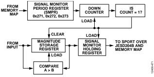
Figure 98. Signal Monitor Block
