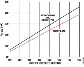
Figure 76. I<sub>AVDD3</sub> vs. Buffer Current Setting in Register 0x018
