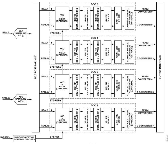
Figure 102. DDC Detailed Block Diagram
