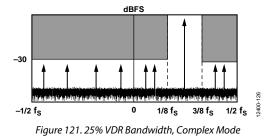
The center frequency  $(f_{VDR})$  of the VDR function can be tuned within the Nyquist band from 0 to 15/16 f<sub>s</sub> in 1/16 f<sub>s</sub> steps. In complex mode, Tuning Word 0 (0x00) through Tuning Word 15 (0x0F) are valid. Table 29 and Table 30 show the tuning words and frequency values for the 25% complex mode. Table 29 shows the relative frequency values, and Table 30 shows the absolute frequency values based on a sample rate of 737.28 MSPS.
