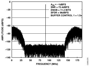
Figure 117. AD6674-750, f<sub>CLOCK</sub> = 750 MHz, f<sub>S</sub> = 375 MSPS, f<sub>IN</sub> = 90.3 MHz, 28% BW Mode, Tuning Word = 19 (f<sub>S</sub>/4 Tuning)
