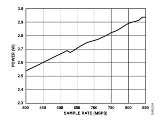
Figure 43. Power Dissipation vs. Sample Rate ( $f_s$ ); L = 4, M = 2, F = 1 for  $f_s \ge 625$  MSPS and L = 2, M = 2, F = 2 for  $f_s < 625$  MSPS (Default SPI)
