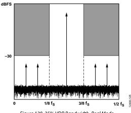
Figure 120. 25% VDR Bandwidth, Real Mode
