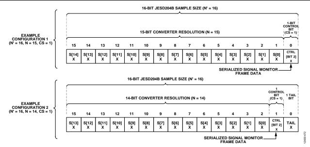
Figure 99. Signal Monitor Control Bit Example Configurations
