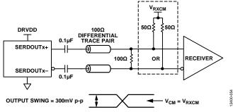
Figure 127. AC-Coupled Digital Output Termination Example
