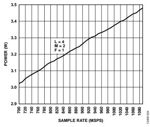
Figure 24. Power Dissipation vs. Sampel Rate (fs) (Default SPI)
