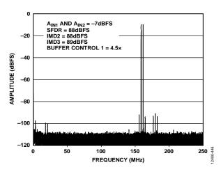
Figure 57. Two-Tone FFT;  $f_{IN1} = 338 \text{ MHz}$ ,  $f_{IN2} = 341 \text{ MHz}$
