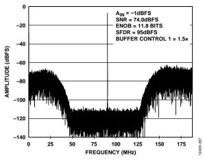
Figure 114. AD6674-750,  $f_{clock} = 750 \text{ MHz}$ ,  $f_s = 375 \text{ MSPS}$ ,  $f_{IN} = 90.3 \text{ MHz}$ , 21% BW Mode, Tuning Word = 26 ( $f_s/4$  Tuning)
