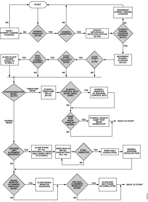
Figure 142. Multichip Synchronization
