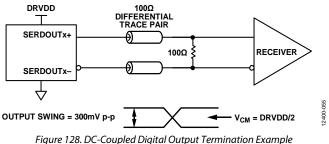
If there is no far-end receiver termination, or if there is poor differential trace routing, timing errors may result. To avoid such timing errors, it is recommended that the trace length be less than six inches, and that the differential output traces be close together and at equal lengths.
