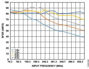
Figure 84. Buffer Current Sweeps, AD6674-500 (SFDR vs. Input Frequency and  $I_{BUFF}$ ); 10 MHz < f<sub>IN</sub> < 450 MHz; Front-End Network Shown in Figure 74
