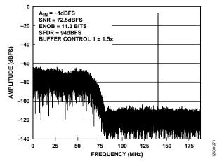
Figure 118. AD6674-750, f<sub>CLOCK</sub> = 750 MHz, f<sub>S</sub> = 375 MSPS, f<sub>IN</sub> = 140.3 MHz, 28% BW Mode, Tuning Word = 43
