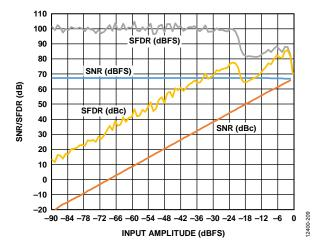
Figure 22. SNR/SFDR vs. Input Amplitude ( $A_{IN}$ ),  $f_{IN} = 170.3$  MHz
