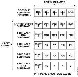
Figure 100. SPORT over JESD204B Signal Monitor Frame Data
