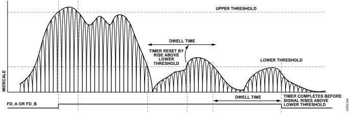
Figure 97. Threshold Settings for FD\_A and FD\_B Signals
