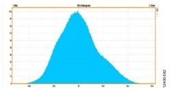
Figure 133. Histogram, External 100  $\Omega$  Terminations at 7.37 Gbps
