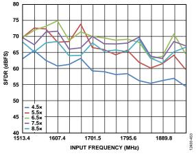
Figure 79. Buffer Current Sweeps, AD6674-1000 (SFDR vs. Input Frequency and  $I_{BUFF}$ ); 1500 MHz < f<sub>IN</sub> < 2 GHz; Front-End Network Shown in Figure 74
