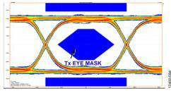
Figure 135. Digital Output Data Eye, External 100  $\Omega$  Terminations at 6 Gbps
