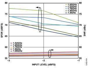
Figure 80. SNR/SFDR vs. Input Level and Input Frequencies, AD6674-1000
