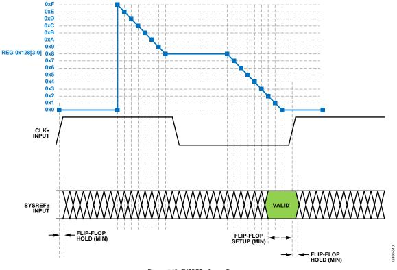
Figure 143. SYSREF± Setup Detector
