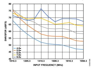
Figure 86. Buffer Current Sweeps, AD6674-500 (SFDR vs. Input Frequency and  $I_{\it BUFF}$ ); 1 GHz <  $f_{\rm IN}$  < 2 GHz; Front-End Network Shown in Figure 74
