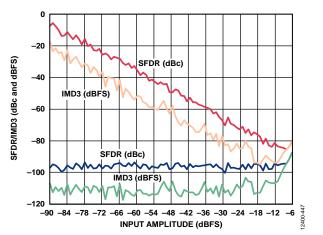
Figure 58. Two-Tone SFDR/IMD3 vs. Input Amplitude (A\_{IN}) with  $f_{\rm IN1}$  = 184 MHz and  $f_{\rm IN2}$  = 187 MHz
