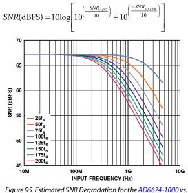
Figure 95. Estimated SNR Degradation for the AD6674-1000 vs. Input Frequency and Jitter
