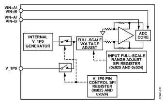
Figure 87. Internal Reference Configuration and Controls
