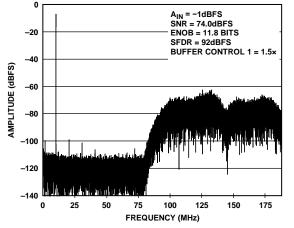
Figure 113. AD6674-750,  $f_{CLOCK} = 750$  MHz,  $f_S = 375$  MSPS,  $f_{IN} = 10.3$  MHz, 21% BW Mode, Tuning Word = 0
