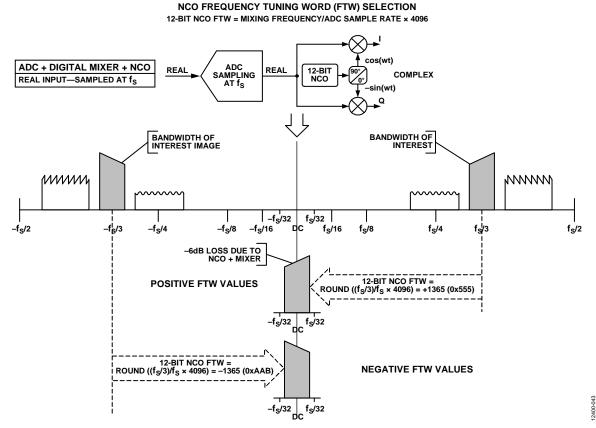
Figure 104. DDC NCO Frequency Tuning Word Selection—Real Inputs
