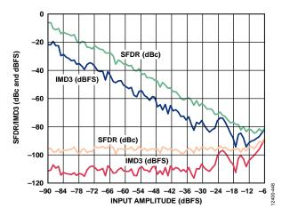
Figure 59. Two-Tone SFDR/IMD3 vs. Input Amplitude (A<sub>IN</sub>) with  $f_{IN1} = 338$  MHz and  $f_{IN2} = 341$  MHz
