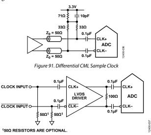
Figure 92. Differential LVDS Sample Clock
