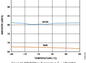
Figure 42. SNR/SFDR vs. Temperature,  $f_{IN} = 170.3 \text{ MHz}$
