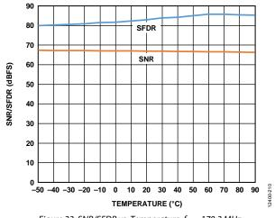
Figure 23. SNR/SFDR vs. Temperature,  $f_{IN} = 170.3$  MHz
