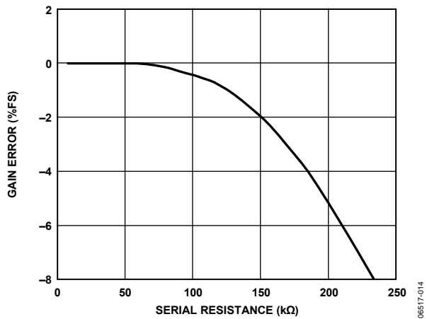
Figure 14. Capacitance Input Gain Error vs. Serial Resistance, V_{DD} = 3.3\text{ V} , CIN to EXC = 2 pF
