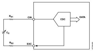
Figure 45. Parasitic Serial Resistance
