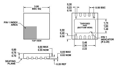
\*FOR PROPER CONNECTION OF THE EXPOSED PAD PLEASE REFER TO THE PIN CONFIGURATION AND FUNCTION DESCRIPTIONS SECTION OF THIS DATA SHEET.
