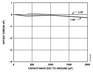
Figure 7. Capacitance Input Offset Error vs. Capacitance EXC to GND,  $V_{DD} = 1.8 \text{ V}$  and 3.3 V, CIN Pin Open Circuit
