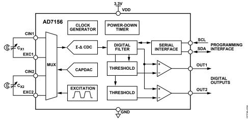
Figure 22. AD7156 Block Diagram
