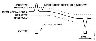
Figure 27. In-Window (Adaptive) Threshold Mode
