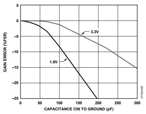
Figure 6. Capacitance Input Gain Error vs. Capacitance CIN to GND,  $V_{\rm DD}=1.8~V$  and 3.3 V, CIN to EXC = 9 pF
