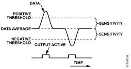
Figure 30. Threshold Sensitivity
