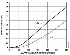
Figure 4. Capacitance Input Offset Error vs. Capacitance CIN to GND,  $V_{\text{DD}}$  = 1.8 V and 3.3 V, EXC Pin Open Circuit
