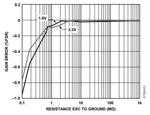
Figure 12. Capacitance Input Gain Error vs. Resistance EXC to GND,  $V_{\rm DD}=1.8~V$  and 3.3 V, CIN to EXC = 3 pF
