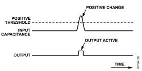
Figure 25. Positive Threshold Mode Indicates Positive Change in Input Capacitance
