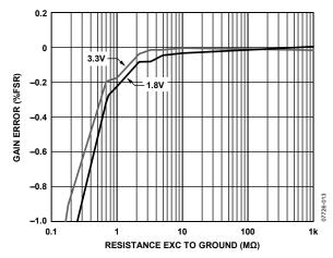
Figure 13. Capacitance Input Gain Error vs. Resistance EXC to GND,  $V_{DD} = 1.8 \text{ V}$  and 3.3 V, CIN to EXC = 9 pF
