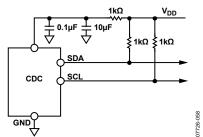
Figure 48. AD7156 VDD Decoupling and Filtering
