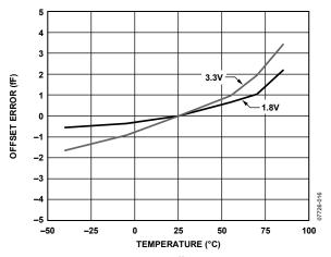
Figure 16. Capacitance Input Offset Error vs. Temperature,  $V_{DD} = 1.8 \ V$  and 3.3 V, CIN and EXC Pins Open Circuit
