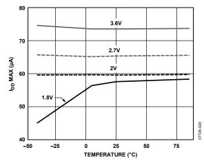
Figure 20. Current vs. Temperature,  $V_{DD} = 1.8 \text{ V}, 2 \text{ V}, 2.7 \text{ V}, \text{ and } 3.6 \text{ V}$
