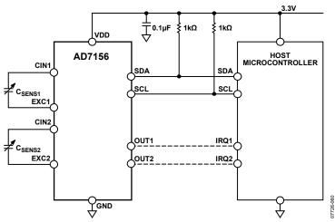
Figure 50. AD7156 Interfaced to a Host Microcontroller
