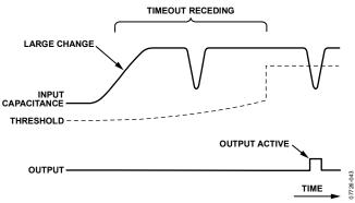
Figure 35. Positive Timeout in Negative Threshold Mode Shortens Period of Missing Output Trigger
