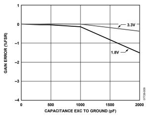
Figure 9. Capacitance Input Gain Error vs. Capacitance EXC to GND,  $V_{\rm DD}=1.8~V$  and 3.3~V, CIN to EXC = 9~pF
