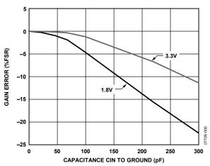
Figure 5. Capacitance Input Gain Error vs. Capacitance CIN to GND,  $V_{\rm DD}=1.8~V$  and 3.3 V, CIN to EXC = 3 pF
