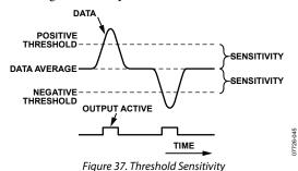
The sensitivity is an 8-bit value and is mapped to the lower eight bits of the 12-bit CDC data, that is, it corresponds to the 16-bit data register as shown in Figure 38.
