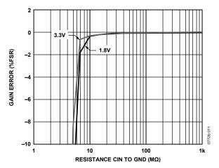
Figure 11. Capacitance Input Gain Error vs. Resistance CIN to GND,  $V_{\rm DD}=1.8~V$  and 3.3 V, CIN to EXC = 9 pF
