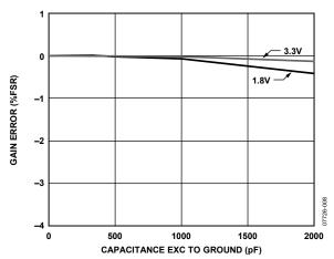
Figure 8. Capacitance Input Gain Error vs. Capacitance EXC to GND,  $V_{DD} = 1.8 \text{ V}$  and 3.3 V, CIN to EXC = 3 pF
