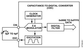
Figure 23. CDC Simplified Block Diagram
