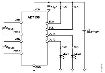
Figure 49. AD7156 Standalone Operation Application Diagram
