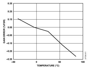
Figure 17. Capacitance Input Gain Error vs. Temperature,  $V_{DD} = 2.7 \text{ V}$ , CIN to EXC = 4 pF
