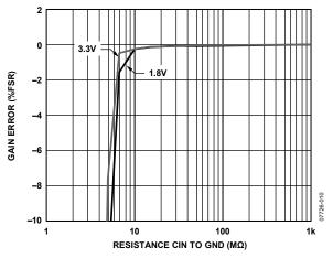
Figure 10. Capacitance Input Gain Error vs. Resistance CIN to GND,  $V_{\rm DD}$  = 1.8 V and 3.3 V, CIN to EXC = 3 pF
