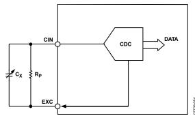
Figure 44. Parasitic Parallel Resistance
