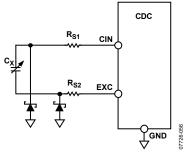
Figure 46. AD7156 CIN Overvoltage Protection
