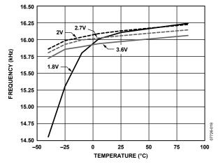
Figure 18. EXC Frequency Error vs. Temperature,  $V_{\rm DD} = 1.8 \text{ V}$ , 2 V, 2.7 V, and 3.6 V
