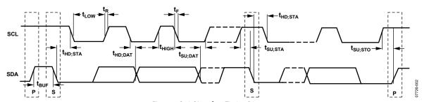
Figure 2. Serial Interface Timing Diagram
