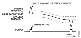
Figure 28. Out-Window (Adaptive) Threshold Mode
