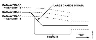
Figure 33. Threshold Timeout After a Large Change in CDC Data
