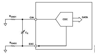
Figure 43. Parasitic Resistance to Ground
