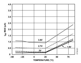
Figure 21. Power-Down Current vs. Temperature,  $V_{DD} = 1.8 V, 2 V, 2.7 V, and 3.6 V$
