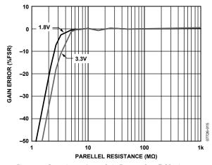
Figure 15. Capacitance Input Gain Error vs. Parallel Resistance,  $V_{\rm DD} = 1.8$  V and 3.3 V, CIN to EXC = 3 pF
