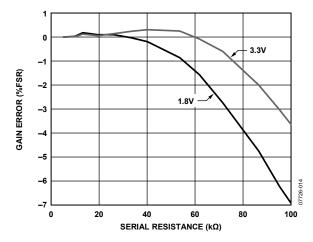
Figure 14. Capacitance Input Gain Error vs. Serial Resistance,  $V_{DD} = 1.8 \text{ V}$  and 3.3 V, CIN to EXC = 3 pF
