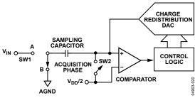
Figure 20. ADC Conversion Phase
