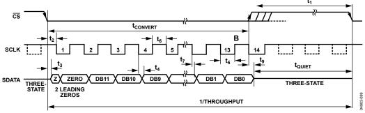
Figure 31. AD7276 Serial Interface Timing Diagram 14 SCLK Cycle
