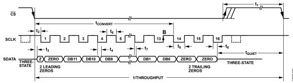
Figure 32. AD7276 Serial Interface Timing Diagram 16 SCLK Cycle
