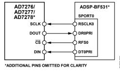
Figure 36. Interfacing with the ADSP-BF531
