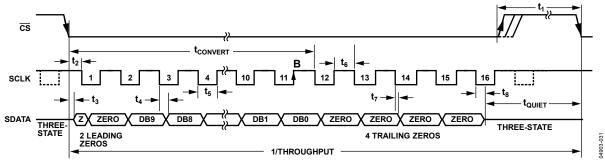
Figure 33. AD7277 Serial Interface Timing Diagram
