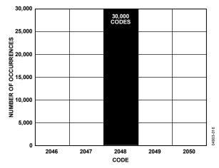
Figure 14. Histogram of Codes for 30,000 Samples
