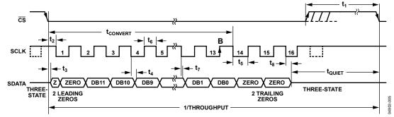
Figure 5. AD7276 Serial Interface Timing Diagram
