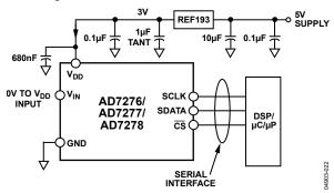
Figure 22. REF193 as Power Supply to the AD7276/AD7277/AD7278
