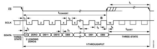
Figure 6. AD7276 Serial Interface Timing 14 SCLK Cycle
