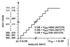
Figure 21. AD7276/AD7277/AD7278 Transfer Characteristics
