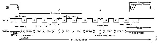
Figure 34. AD7278 Serial Interface Timing Diagram
