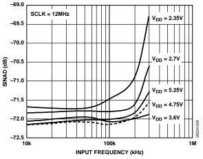
Figure 5. AD7476-EP SINAD vs. Input Frequency at 605 kSPS
