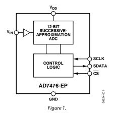
The reference for the part is taken internally from  $V_{DD}$ . This allows the widest dynamic input range to the ADC. Thus, the analog input range for the part is 0 V to  $V_{DD}$ . The conversion rate is determined by the SCLK pin.
