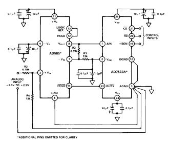
Figure 24. AD7572A-AD585 Sample-and-Hold Interface
