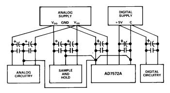
Figure 15. Power Supply Grounding Practice
