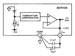
Figure 7. AD7572A Internal -5.25 V Reference
