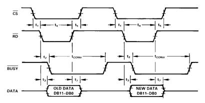
Figure 19. ROM Mode, Parallel Read Timing Diagram
