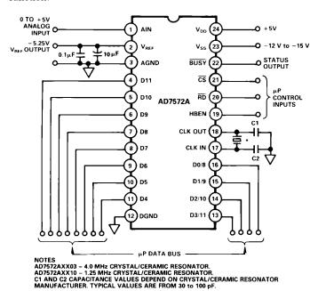
Figure 3. AD7572A Operational Diagram
