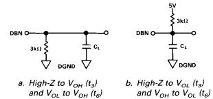
Figure 1. Load Circuits for Access Time
