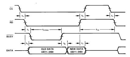
Figure 17. Slow Memory Mode, Parallel Read Timing Diagram
