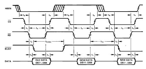
Figure 20. ROM Mode, Two Byte Read Timing Diagram
