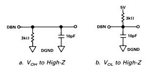
Figure 2. Load Circuits for Output Float Delay
