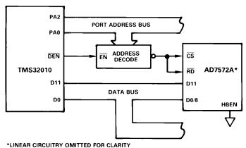
Figure 23. AD7572A-TMS32010 Interface
