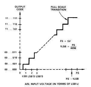
Figure 8. AD7572A Ideal Input/Output Transfer Characteristic
