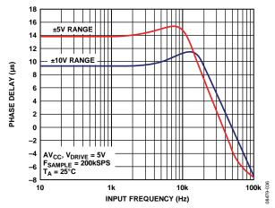
Figure 38. Analog Antialias Filter Phase Response
