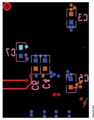
Figure 63. Bottom Layer Decoupling
