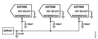
Figure 41. Single External Reference Driving Multiple AD7606/AD7606-6/ AD7606-4 REFIN Pins
