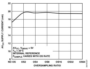
Figure 32. Supply Current vs. Oversampling Rate
