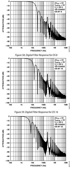
Figure 60. Digital Filter Response for OS 32
