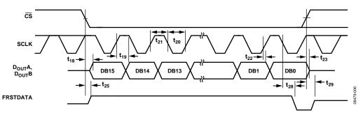
Figure 6. Serial Read Operation (Channel 1)
