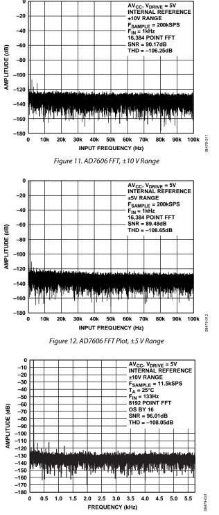
Figure 13. FFT Plot Oversampling By 16, ±10 V Range
