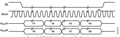
Figure 46. AD7606 Serial Interface with Two Dout Lines
