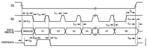
Figure 4. Parallel Mode, Separate  $\overline{CS}$  and  $\overline{RD}$  Pulses
