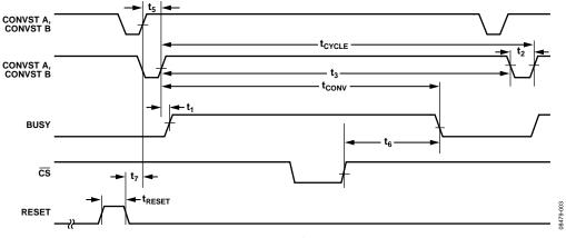
Figure 3. CONVST Timing—Reading During a Conversion
