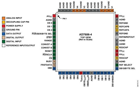
Figure 10. AD7606-4 Pin Configuration
