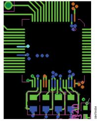
Figure 62. Top Layer Decoupling REFIN/REFOUT, REFCAPA, REFCAPB, and REGCAP Pins
