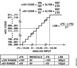
Figure 39. AD7606/AD7606-6/AD7606-4 Transfer Characteristics
