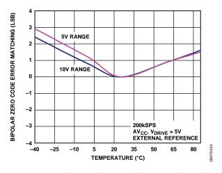
Figure 23. Bipolar Zero Code Error Matching Between Channels
