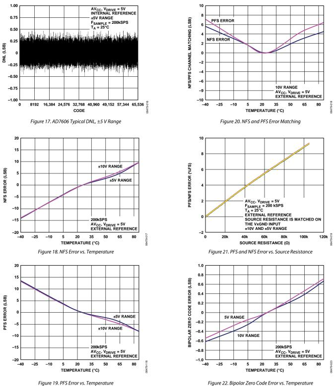
Figure 22. Bipolar Zero Code Error vs. Temperature
