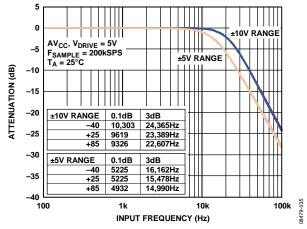
Figure 37. Analog Antialiasing Filter Frequency Response
