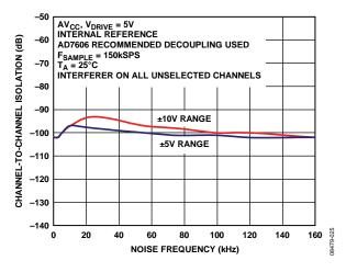
Figure 28. Channel-to-Channel Isolation
