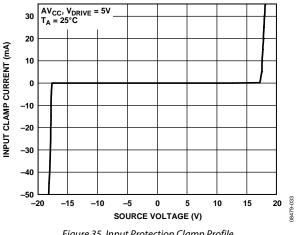
Figure 35. Input Protection Clamp Profile
