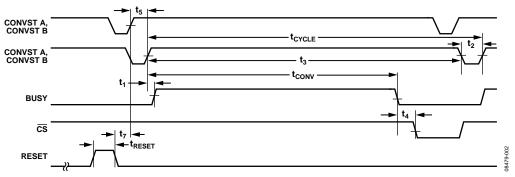
Figure 2. CONVST Timing—Reading After a Conversion
