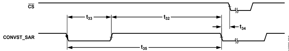
Figure 5. SAR ADC Timing Diagram
