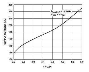
Figure 5. Supply Current vs.  $+V_{CC}$
