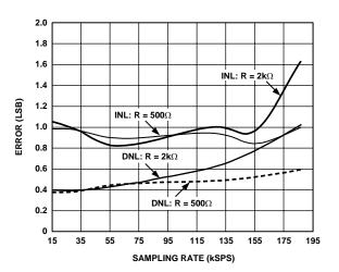
Figure 12. Maximum Sampling Rate vs. R<sub>IN</sub>
