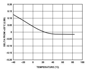
Figure 6. Change in Gain vs. Temperature
