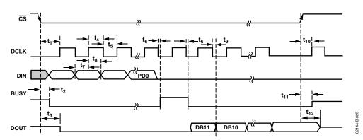
Figure 25. Detailed Timing Diagram
