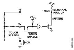
Figure 28. PENIRQ Functional Block Diagram
