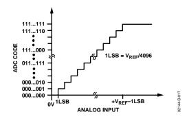
Figure 17. AD7843 Transfer Characteristic
