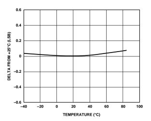
Figure 9. Change in Offset vs. Temperature
