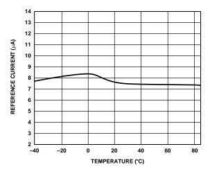
Figure 13. Reference Current vs. Temperature
