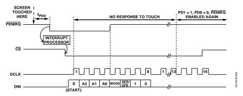
Figure 29. PENIRQ Timing Diagram
