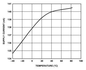
Figure 7. Power-Down Supply Current vs. Temperature
