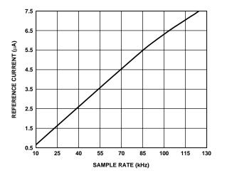
Figure 10. Reference Current vs. Sample Rate
