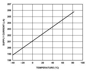
Figure 4. Supply Current vs. Temperature
