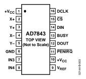
Figure 3. Pin Configuration QSOP/TSSOP
