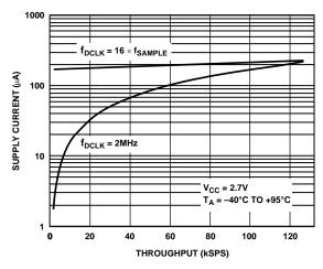
Figure 23. Supply Current vs. Throughput (μA)
