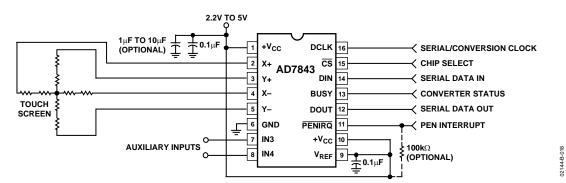
Figure 18. Typical Application Circuit
