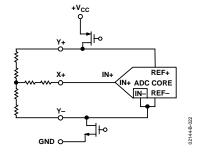
Figure 22. Differential Reference Mode (SER/ $\overline{DFR} = 0$ )
