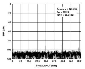
Figure 15. Auxiliary Channel Dynamic Performance (f<sub>SAMPLE</sub> =125 kHz, f<sub>INPUT</sub> = 15 kHz)
