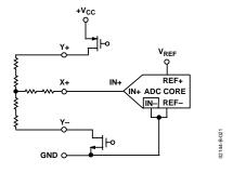
Figure 21. Single-Ended Reference Mode (SER/ $\overline{DFR} = 1$ )
