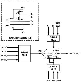
Figure 19. Equivalent Analog Input Circuit
