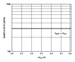
Figure 8. Maximum Sample Rate vs. +V<sub>CC</sub>
