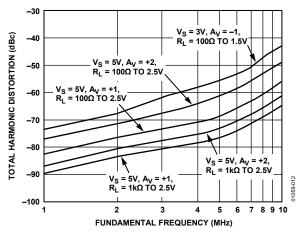
Figure 12. Total Harmonic Distortion vs. Frequency
