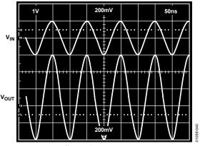
Figure 40. Differential Driver Frequency Response
