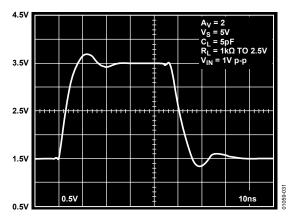
Figure 31. 1 V Pulse Response,  $V_{\rm S} = 5 V$
