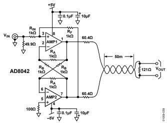
Figure 39. Single-Ended-to-Differential Twisted Pair Line Driver
