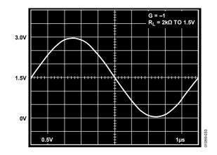
Figure 33. Rail-to-Rail Output Swing,  $V_S = 3 V$
