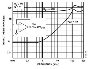
Figure 19. Output Resistance vs. Frequency
