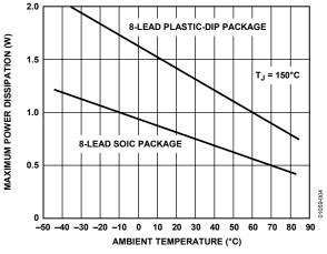
Figure 4. Maximum Power Dissipation vs. Temperature
