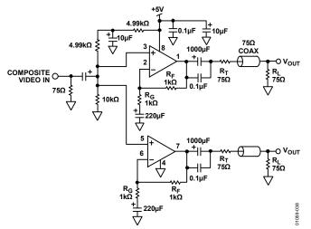
Figure 38. Single-Supply Composite Video Line Driver Using AD8042
