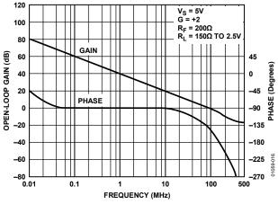
Figure 16. Open-Loop Gain and Phase vs. Frequency
