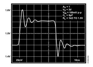
Figure 34. 100 mV Pulse Response,  $V_s = 3 V$
