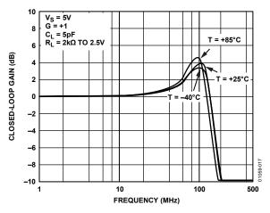
Figure 17. Closed-Loop Frequency Response vs. Temperature
