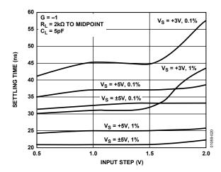
Figure 20. Settling Time vs. Input Voltage
