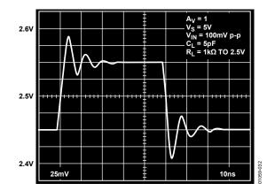
Figure 32. 100 mV Pulse Response,  $V_S = 5 V$
