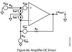
$\overline{Ven}$ ,  $\overline{IN+}$ , and  $\overline{IN-}$  are due to the amplifier.  $V_{R_F}$ ,  $V_{R_G}$ , and  $V_{R_S}$  are due to the feedback network resistors,  $R_G$  and  $R_F$ , and the source resistor,  $R_S$ . The total output voltage noise,  $\overline{V_{OUT\_EN}}$ , is the rms sum of all the contributions.
