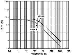
Figure 44. PSRR vs. Frequency
