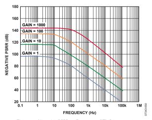
Figure 15. Negative PSRR vs. Frequency, RTI, G = 1 to 1000
