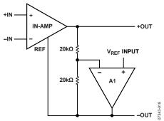
Figure 64. Differential Output Configuration Using an Op Amp
