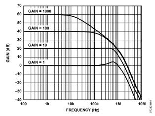
Figure 17. Gain vs. Frequency, G = 1 to 1000
