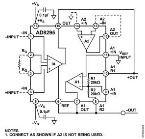
Figure 65. Minimum Component Connections for Differential Output
