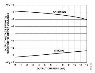
Figure 23. Output Voltage Swing vs. Output Current, G = 1
