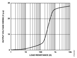
Figure 22. Output Voltage Swing vs. Load Resistance
