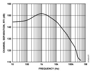
Figure 54. Channel Separation vs. Frequency (Source Channel: In-Amp with  $R_L=2~k\Omega,~G=1$ ; Receive Channel: Op Amp at G=1000)
