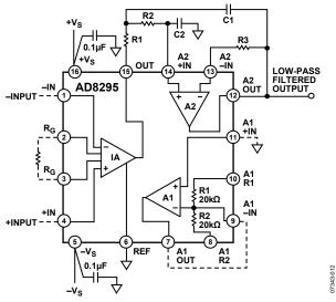
Figure 69. Two-Pole Sallen-Key Filter
