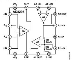
Figure 58. Functional Block Diagram
