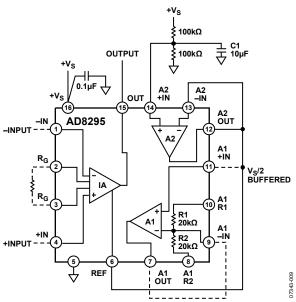
Figure 67. Single-Supply Connection with Buffered Reference
