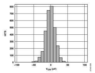
Figure 4. Typical Distribution of Input Offset Voltage
