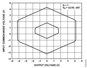
Figure 7. Input Common-Mode Voltage Range vs. Output Voltage, G=1,  $V_S=\pm 2.5$  V,  $v_{REF}=0$  V
