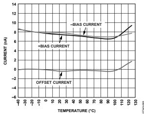
Figure 50. Input Bias Current and Input Offset Current vs. Temperature
