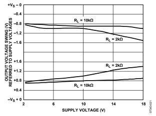
Figure 21. Output Voltage Swing vs. Supply Voltage, G = 1
