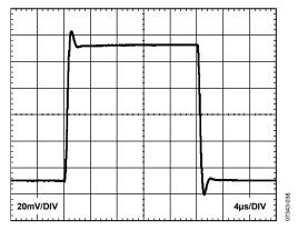
Figure 37. Small Signal Pulse Response, G = 10,  $R_L = 2$   $k\Omega$ ,  $C_L = 100$  pF
