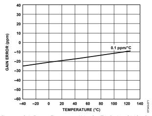
$\label{eq:Figure 52.} \textit{Gain Error vs. Temperature Using On-Chip Resistor Divider, G=2}$
