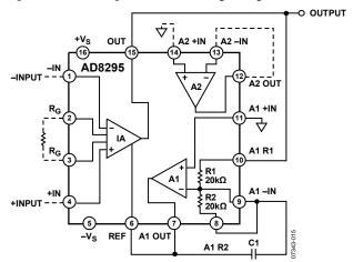
Figure 70. AC-Coupled Connection
