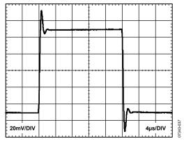
Figure 36. Small Signal Pulse Response, G = 1,  $R_L = 2 k\Omega$ ,  $C_L = 100 pF$
