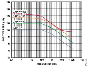
Figure 14. Positive PSRR vs. Frequency, RTI, G = 1 to 1000
