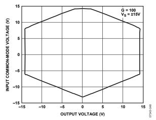
Figure 10. Input Common-Mode Voltage Range vs. Output Voltage,  $G=100,\,V_S=\pm15\,V,\,V_{REF}=0\,V$
