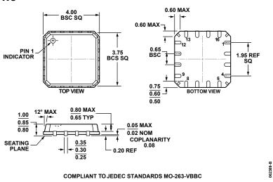
Figure 72. 16-Lead Lead Frame Chip Scale Package [LFCSP\_VQ] 4 mm × 4 mm Body, Very Thin Quad, with Hidden Paddle (CP-16-19) Dimensions shown in millimeters
