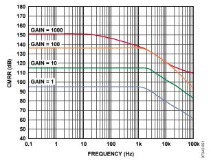
Figure 18. CMRR vs. Frequency, RTI, G = 1 to 1000
