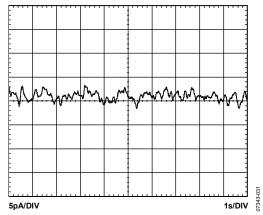
Figure 30. 0.1 Hz to 10 Hz Current Noise
