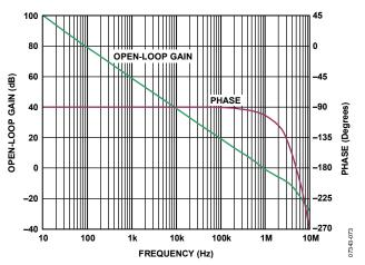
Figure 42. Open-Loop Gain and Phase vs. Frequency,  $C_L = 5 pF$
