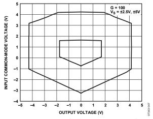
Figure 9. Input Common-Mode Voltage Range vs. Output Voltage, G = 100,  $V_S = \pm 2.5$  V,  $V_{REF} = 0$  V
