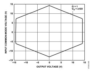
Figure 8. Input Common-Mode Voltage Range vs. Output Voltage, G = 1,  $V_S = \pm 15$  V,  $V_{REF} = 0$  V
