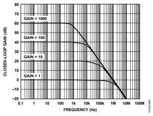
Figure 43. Closed-Loop Gain vs. Frequency, G = 1 to 1000
