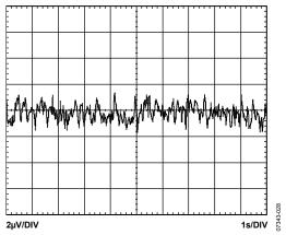
Figure 27. 0.1 Hz to 10 Hz RTI Voltage Noise, G = 1
