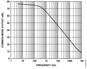
Figure 56. Differential Output Configuration, Common-Mode Output vs. Frequency
