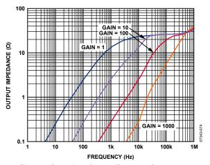
Figure 45. Output Impedance vs. Frequency, G = 1 to 1000
