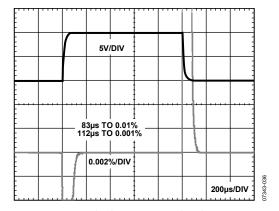
Figure 35. Large Signal Pulse Response and Settling Time, G=1000
