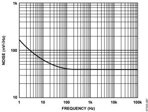
Figure 47. Voltage Noise Density vs. Frequency
