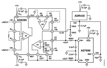
Figure 71. Driving a Differential ADC
