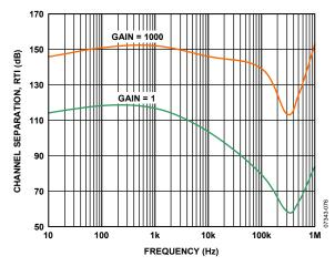
Figure 53. Channel Separation vs. Frequency (Source Channel: Op Amp with  $R_L=2~k\Omega$ ; Receive Channel: In-Amp at G = 1 and G = 1000)
