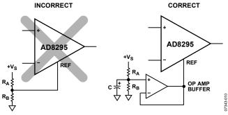
Figure 60. Driving the Reference Pin
