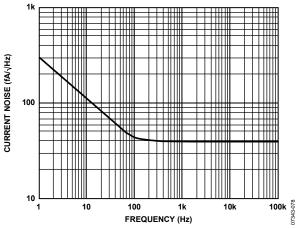
Figure 49. Current Noise Density vs. Frequency
