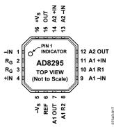
Figure 2. Pin Configuration
