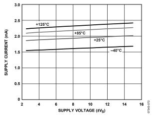
Figure 57. Supply Current vs. Supply Voltage
