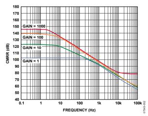
Figure 19. CMRR vs. Frequency, RTI, 1 k $\Omega$  Source Imbalance, G=1 to 1000
