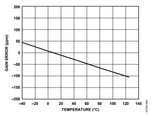
Figure 16. Gain Error vs. Temperature, G = 1
