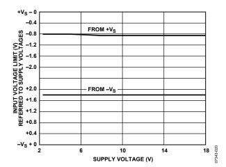
Figure 20. Input Voltage Limit vs. Supply Voltage, G = 1
