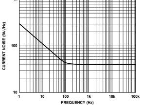
Figure 29. Current Noise Spectral Density vs. Frequency
