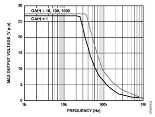
Figure 31. Large Signal Frequency Response
