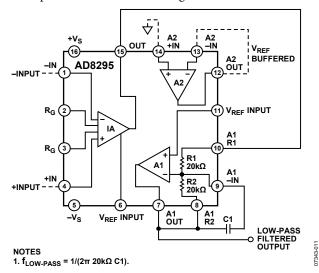
Figure 68. Single-Pole Output Filter Using a Single External Capacitor
