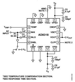
Figure 23. Basic Connections
