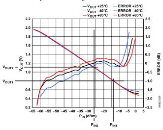
Figure 33. Output Voltage and Error vs.  $P_{IN}$  with 2-Point Calibration at -10 dBm and -30 dBm
