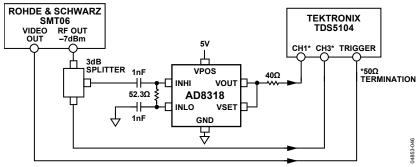
Figure 47. Pulse Response Measurement Test Setup
