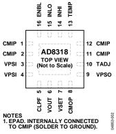
Figure 3. Pin Configuration
