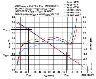
Figure 32. Transfer Function at 2.2 GHz
