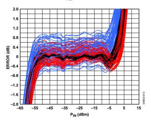
Figure 14. Distribution of Error at Temperature After Ambient Normalization vs. Input Amplitude at 5.8 GHz for at Least 70 Devices,  $R_{TADJ} = 1000 \, \Omega$
