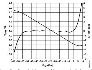
$\textit{Figure 2. Typical Logarithmic Response and Error vs. Input Amplitude at 5.8\,GHz}$
