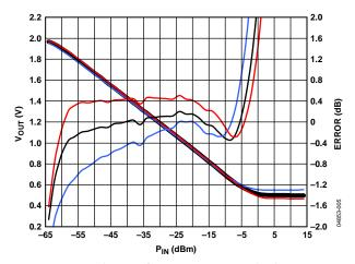
Figure 6. V<sub>OUT</sub> and Log Conformance vs. Input Amplitude at 2.2 GHz, Typical Device
