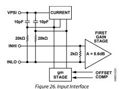
While the input can be reactively matched, this is typically not necessary. An external 52.3  $\Omega$  shunt resistor (connected on the signal side of the input coupling capacitors, see Figure 23) combines with the relatively high input impedance to provide an adequate broadband 50  $\Omega$  match.
