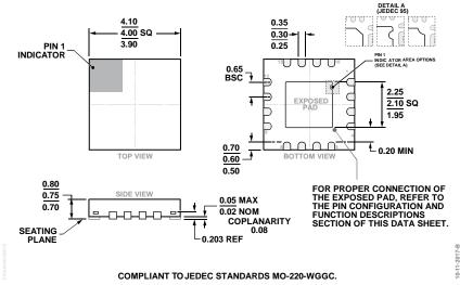
Figure 51. 16-Lead Lead Frame Chip Scale Package [LFCSP] 4 mm × 4 mm Body and 0.75 mm Package Height (CP-16-23) Dimensions shown in millimeters
