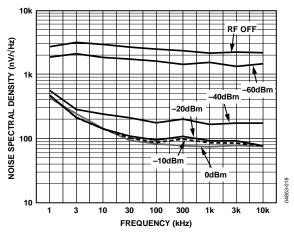
Figure 19. Noise Spectral Density of Output; CLPF = Open
