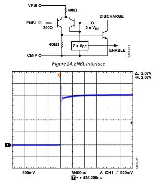
Figure 25. ENBL Response Time; VPOS = 5.0 V; Input AC-Coupling Caps = 18 pF; CLPF = Open
