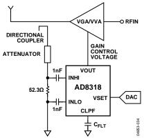
Figure 42. AD8318 Controller Mode
