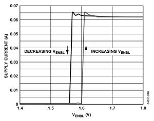
Figure 17. Supply Current vs. Enable Voltage
