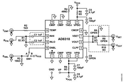
Figure 48. Evaluation Board Schematic
