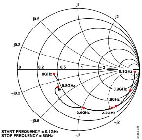
Figure 16. Input Impedance vs. Frequency; No Termination Resistor on INHI,  $Z_0 = 50\,\Omega$
