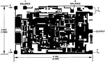
SUBSTRATE CONNECTED TO + Vs
