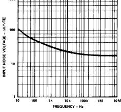
Figure 17. Input Noise Voltage Spectral Density
