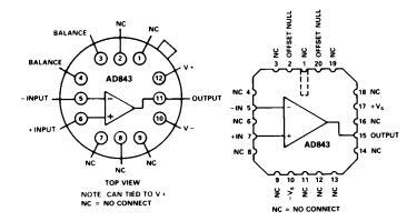
The AD843 is offered in either 8-pin plastic DIP or hermetic cerdip packages, in 16-pin SOIC, 20-Pin LCC, or in a 12-pin metal can. Chips are also available.
