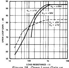
Figure 19. Open Loop Gain vs. Resistive Load
