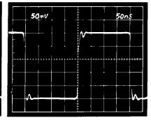
Figure 23c. Buffer Cap Load Small Signal Pulse Response.  $C_F = 33$  pF,  $C_L = 10$  pF
