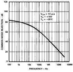
Figure 13. Common Mode Rejection vs. Frequency
