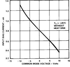
Figure 7. Input Bias Current vs. Common Mode Voltage
