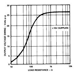
Figure 3. Output Voltage Swing vs. Load Resistance
