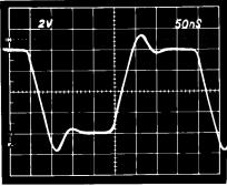
Figure 21b. Inserter Cap Load Large Signal Pulse Response.  $C_F = 15 \text{ pF}, C_L = 410 \text{ pF}$
