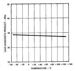
Figure 9. Gain Bandwidth Product vs. Temperature
