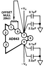
Offset Null Configuration (DIP Pinout)
