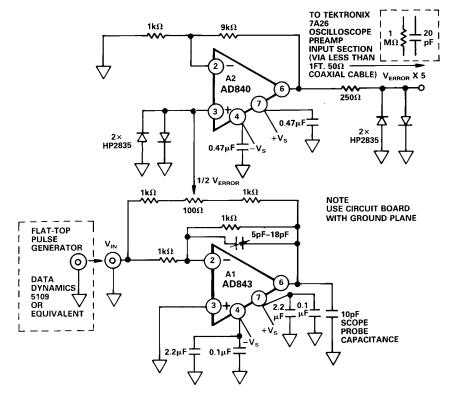
Figure 27. Settling Time Test Circuit
