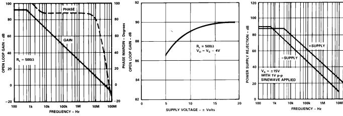
Figure 10. Open Loop Gain and Phase Margin vs. Frequency
