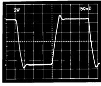
Figure 20b. Inverter Large Signal Pulse Response.  $C_F = 0$ ,  $C_L = 10$  pF
