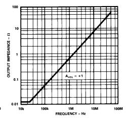
Figure 6. Output Impedance vs. Frequency
