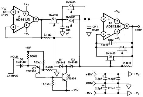
Figure 25. A Fast Switching Sample-and-Hold Amplifier
