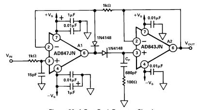
Figure 29. A Fast Peak Detector Circuit
