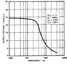
Figure 14. Large Signal Frequency Response
