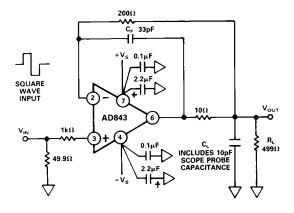
Figure 23a. Unity Gain Buffer Circuit for Driving Capacitive Loads
