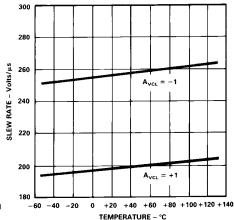
Figure 18. Slew Rate vs. Temperature
