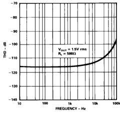
Figure 16. Harmonic Distortion vs. Frequency
