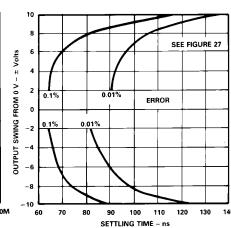
Figure 15. Output Swing and Error vs. Settling Time
