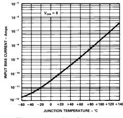
Figure 5. Input Bias Current vs. Junction Temperature
