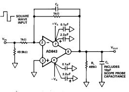
Figure 20a. Inverting Amplifier Connection
