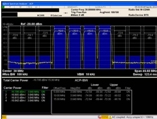
Figure 30. AD9135 Four-Carrier W-CDMA ACLR, f_{OUT} = 30 MHz, f_{DAC} = 1966 MHz, 4\times Interpolation, PLL Frequency = 245 MHz
