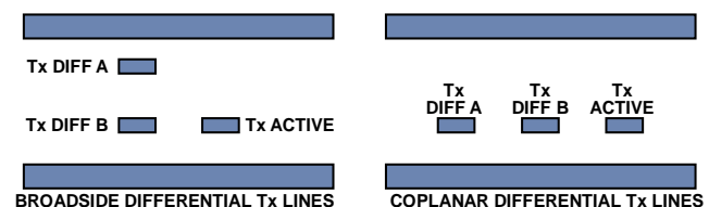
Figure 66. Broadside vs. Coplanar Differential Stripline Routing Techniques
