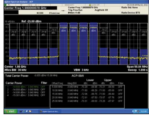
Figure 56. Four-Carrier W-CDMA at 1980 MHz
