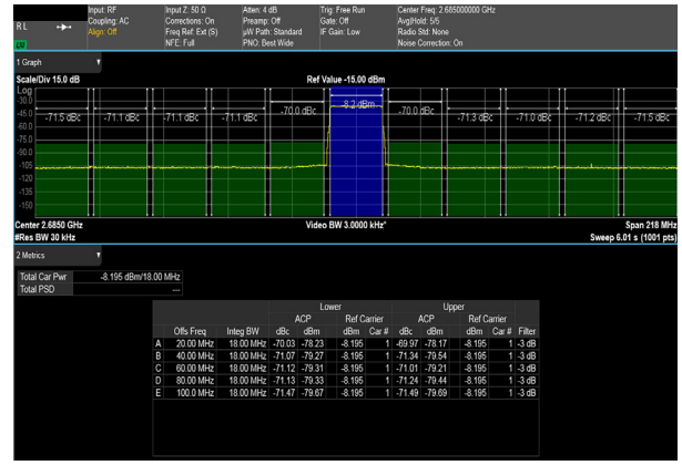
Figure 35. 20 MHz LTE Carrier ACLR at 2685.0 MHz
