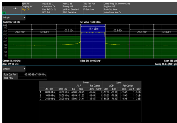
Figure 40. 80 MHz 802.11AC ACLR at 5530.0 MHz
