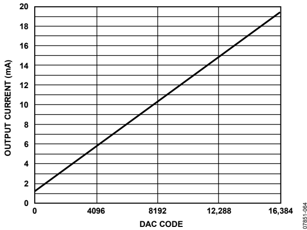
Figure 63. Gain Curve for FSC[9:0] = 512, DAC Offset = 1.228 mA
