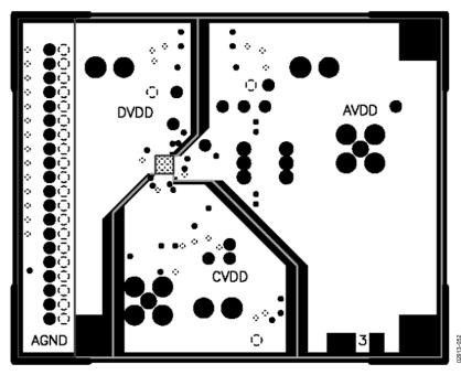
Figure 55. LFCSP Evaluation Board Layout—Power Plane
