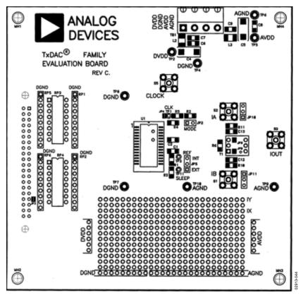
Figure 47. SOIC Evaluation Board Assembly—Primary Side
