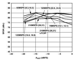
Figure 14. Dual-Tone IMD vs.  $A_{OUT}$  at  $f_{OUT} = f_{CLOCK}/7$
