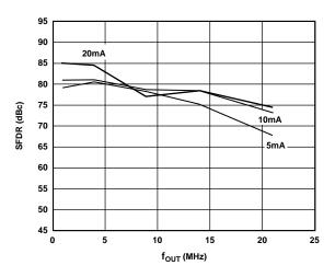
Figure 10. SFDR vs.  $f_{\text{OUT}}$  and  $I_{\text{OUTFS}}$  at 65 MSPS and 0 dBFS
