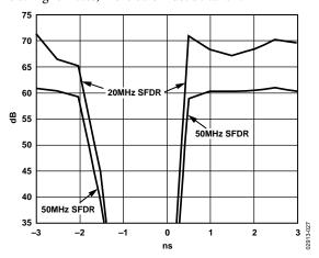
Figure 30. SFDR vs. Clock Placement at  $f_{OUT} = 20$  MHz and 50 MHz
