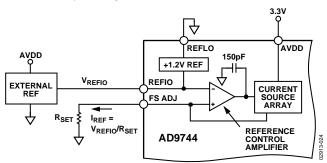
Figure 27. External Reference Configuration
