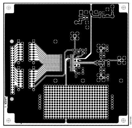
Figure 43. SOIC Evaluation Board—Primary Side
