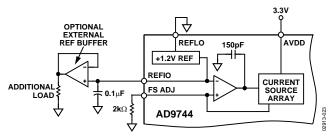
Figure 26. Internal Reference Configuration
