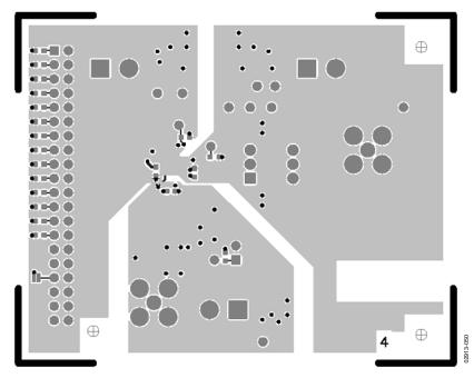
Figure 53. LFCSP Evaluation Board Layout—Secondary Side
