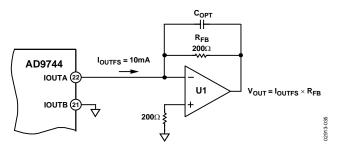
Figure 38. Unipolar Buffered Voltage Output
