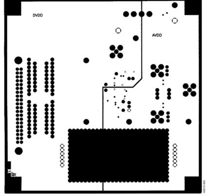
Figure 46. SOIC Evaluation Board—Power Plane
