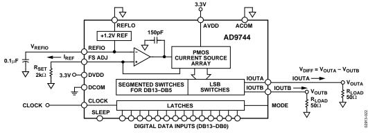
Figure 23. Simplified Block Diagram (SOIC/TSSOP Packages)
