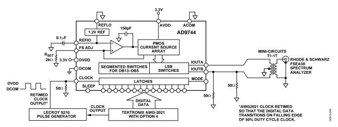
Figure 24. Basic AC Characterization Test Set-Up (SOIC/TSSOP Packages)
