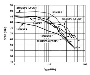
Figure 5. SFDR vs. fout at 0 dBFS
