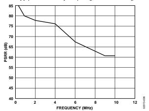
Figure 39. Power Supply Rejection Ratio (PSRR) vs. Frequency
