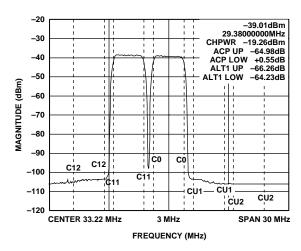
Figure 21. Two-Carrier UMTS Spectrum,  $f_{CLOCK} = 122.88$  MSPS (ACLR = 64 dB) LFCSP Package
