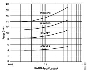
Figure 32. I<sub>DVDD</sub> vs. Ratio at DVDD = 3.3 V
