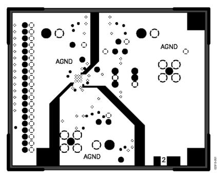
Figure 54. LFCSP Evaluation Board Layout—Ground Plane
