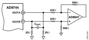
Figure 35. DC Differential Coupling Using an Op Amp
