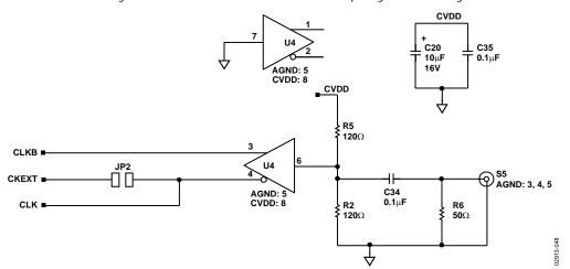
Figure 51. LFCSP Evaluation Board Schematic—Clock Input
