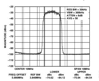
Figure 22. Single-Carrier UMTS Spectrum,  $f_{CLOCK} = 61.44$  MSPS (ACLR = 74 dB) LFCSP Package
