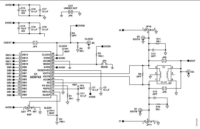
Figure 42. SOIC Evaluation Board—Output Signal Conditioning
