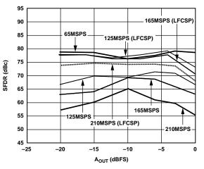
Figure 12. Single-Tone SFDR vs. A<sub>OUT</sub> at  $f_{OUT} = f_{CLOCK}/5$
