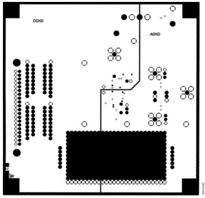
Figure 45. SOIC Evaluation Board—Ground Plane
