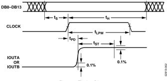
Figure 2. Timing Diagram
