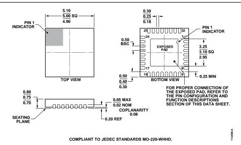
Figure 60. 32-Lead Lead Frame Chip Scale Package [LFCSP\_WQ] 5 mm × 5 mm Body, Very Very Thin Quad (CP-32-7) Dimensions shown in millimeters
