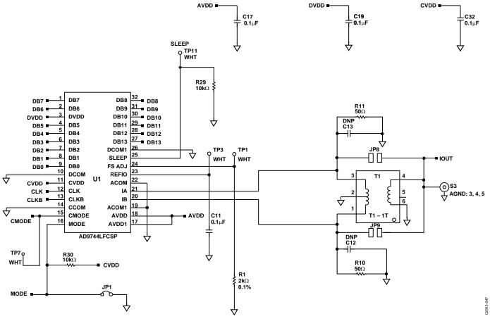
Figure 50. LFCSP Evaluation Board Schematic—Output Signal Conditioning
