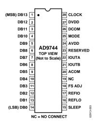
Figure 3. 28-Lead SOIC and TSSOP
