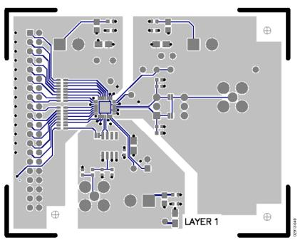
Figure 52. LFCSP Evaluation Board Layout—Primary Side
