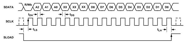
Figure 6. Serial Write Operating Timing
