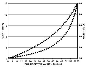
Figure 13. PGA Gain Transfer Function
