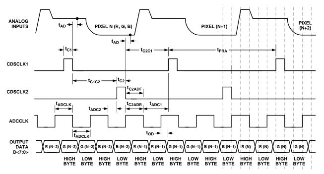
Figure 1. 3-Channel CDS Mode Timing
