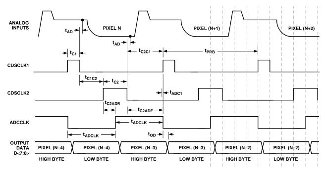
Figure 2. 1-Channel CDS Mode Timing
