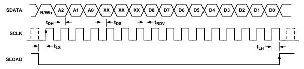
Figure 7. Serial Read Operation Timing
