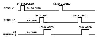
Figure 9. CDS-Mode Internal Switch Timing
