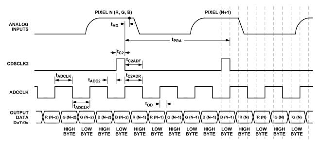
Figure 3. 3-Channel SHA Mode Timing
