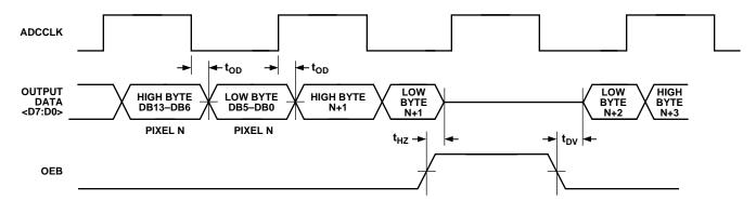
Figure 5. Digital Output Data Timing
