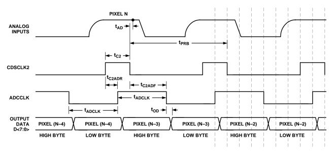
Figure 4. 1-Channel SHA Mode Timing
