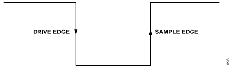
Figure 98. SPI Mode 0 SCLK Edges
