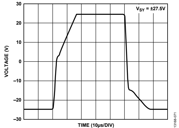
Figure 74. Large Signal Transient Response Example
