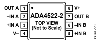
Figure 1. 8-Lead MSOP (RM Suffix) and 8-Lead SOIC (R Suffix) Pin Configuration
