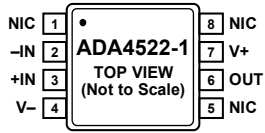
Figure 3. ADA4522-1 Pin Configuration
