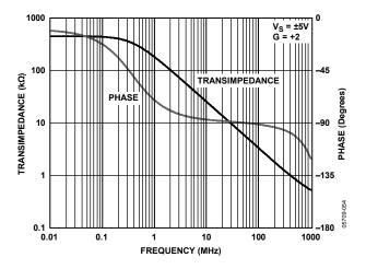
Figure 46. Transimpedance and Phase vs. Frequency
