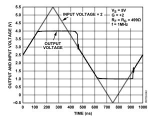
Figure 45. Output Overdrive Recovery
