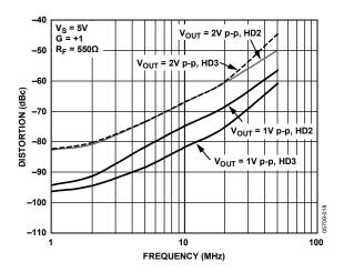
Figure 17. Harmonic Distortion vs. Frequency
