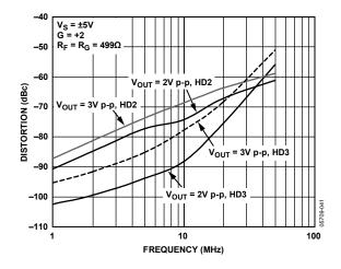
Figure 19. Harmonic Distortion vs. Frequency
