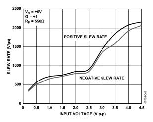
Figure 34. Slew Rate vs. Input Voltage
