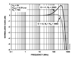
Figure 14. Small Signal Frequency Response for Various Gains
