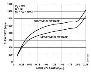
Figure 37. Slew Rate vs. Input Voltage
