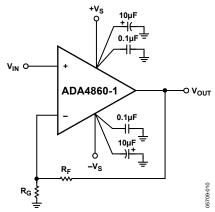
Figure 51. Noninverting Gain
