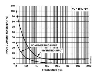
Figure 43. Input Current Noise vs. Frequency
