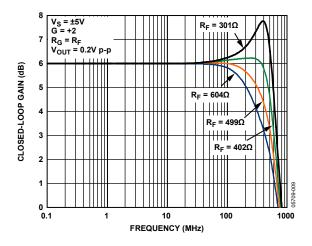
Figure 10. Small Signal Frequency Response vs. R<sub>F</sub>
