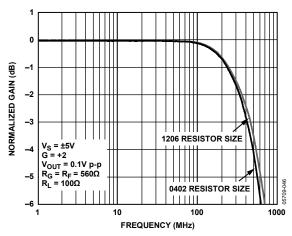
Figure 59. Small Signal Frequency Response vs. Resistor Size
