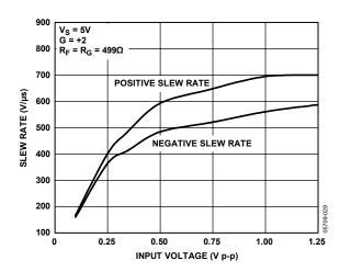
Figure 38. Slew Rate vs. Input Voltage
