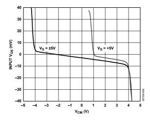
Figure 49. Input Vos vs. Common-Mode Voltage
