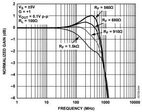
Figure 56. Small Signal Frequency Response vs. R<sub>F</sub>
