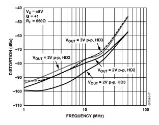
Figure 16. Harmonic Distortion vs. Frequency
