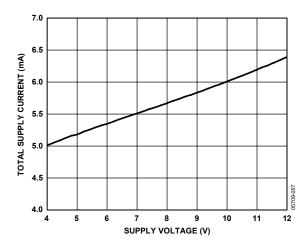
Figure 50. Supply Current vs. Supply Voltage
