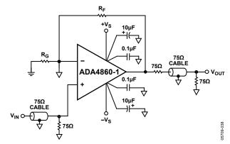
Figure 55. Video Driver Schematic
