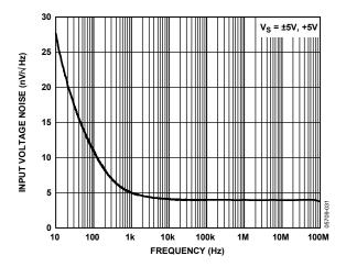
Figure 40. Input Voltage Noise vs. Frequency
