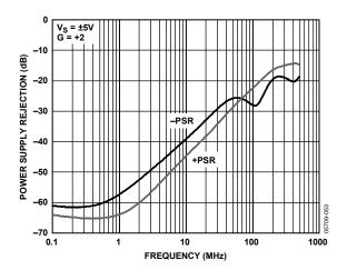
Figure 41. Power Supply Rejection vs. Frequency
