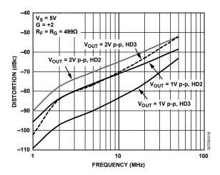
Figure 20. Harmonic Distortion vs. Frequency
