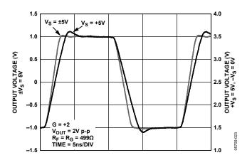
Figure 31. Large Signal Transient Response for Various Supplies
