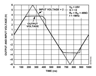
Figure 42. Output Overdrive Recovery
