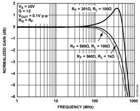
Figure 57. Small Signal Frequency Response vs. R<sub>F</sub> vs. R<sub>L</sub>
