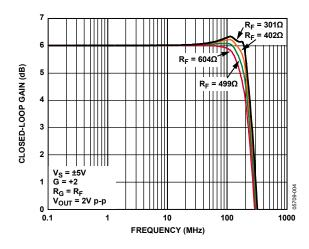
Figure 13. Large Signal Frequency Response vs. R<sub>F</sub>
