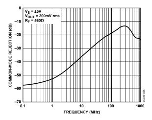
Figure 44. Common-Mode Rejection vs. Frequency
