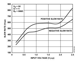
Figure 35. Slew Rate vs. Input Voltage
