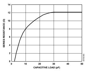
Figure 54. Recommended  $R_{SERIES}$  vs. Capacitive Load
