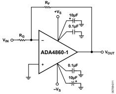
Figure 52. Inverting Gain
