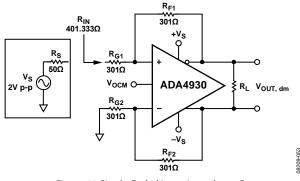
Figure 46. Single-Ended Input Impedance R<sub>IN</sub>
