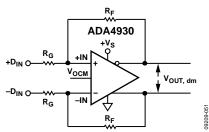
Figure 44. ADA4930-1/ADA4930-2 Configured for Balanced (Differential) Inputs
