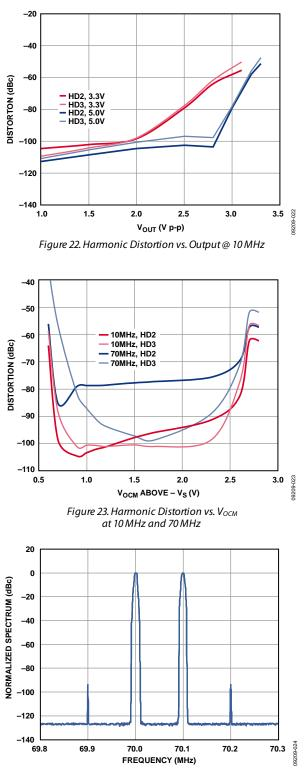
Figure 24. 70 MHz Intermodulation Distortion
