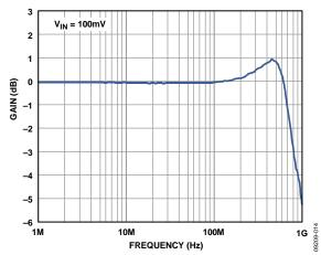
Figure 14. V<sub>OCM</sub> Small Signal Frequency Response
