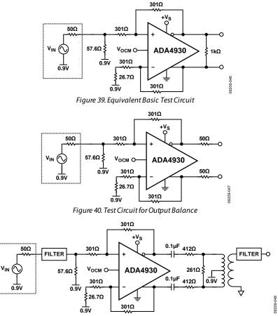
Figure 41. Test Circuit for Distortion Measurements
