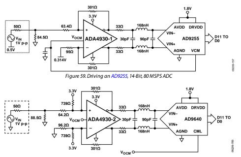
Figure 60. Driving an AD9640, 14-Bit, 80 MSPS ADC
