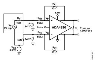
Figure 53. Single-Supply Application Circuit with DC Source Bias
