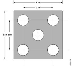
Figure 57. Recommended PCB Thermal Attach Pad Dimensions (Millimeters)
