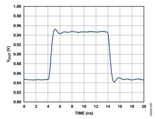
Figure 35. Small Signal V<sub>OCM</sub> Pulse Response
