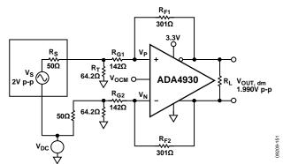
Figure 51. Single-Supply, Terminated Single-Ended-to-Differential System with G = 1
