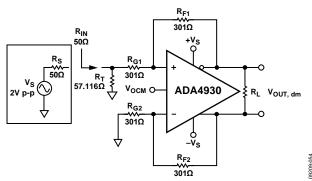
Figure 47. Adding Termination Resistor R<sub>T</sub>
