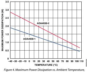
Figure 4. Maximum Power Dissipation vs. Ambient Temperature 4-Layer Board
