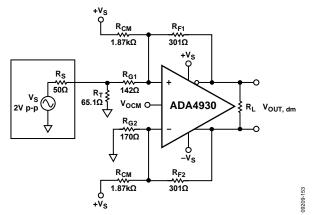
Figure 55. Single-Supply, Single-Ended Input System with Bias Resistors
