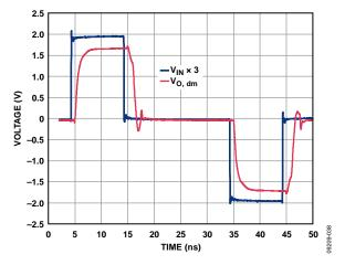
Figure 38. V<sub>o,dm</sub> Overdrive Recovery
