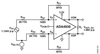
Figure 52. Thevenin Equivalent of Single-Supply Application Circuit
