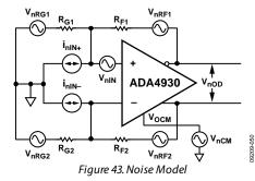
Similar to the case of conventional op amps, the output noise voltage densities can be estimated by multiplying the input-referred terms at +IN and –IN by an appropriate output factor.
