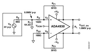
Figure 50. Terminated Single-Ended-to-Differential System with G = 1
