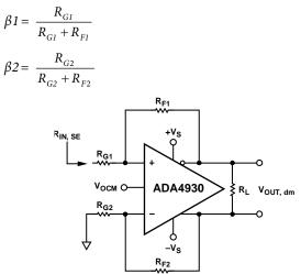
Figure 45. ADA4930-1/ADA4930-2 with Unbalanced (Single-Ended) Input
