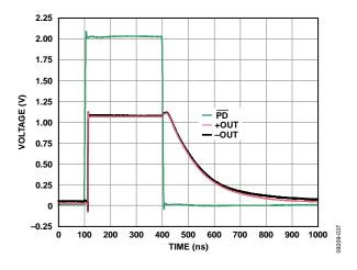
Figure 37. PD Response vs. Time
