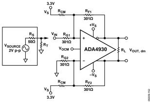
Figure 54. Single-Supply Biasing Scheme with Resistors
