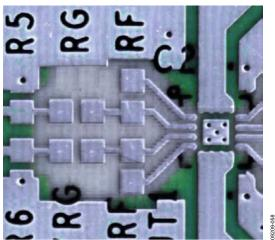
Figure 56. ADA4930-1 Ground and Power Plane Voiding in the Vicinity of R<sub>F</sub> and R<sub>G</sub>
