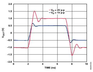
Figure 33. Large Signal Pulse Response
