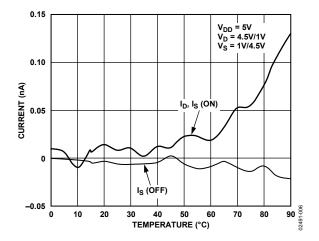
Figure 6. Leakage Currents as a Function of Temperature
