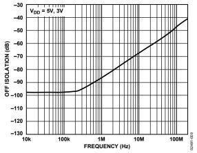
Figure 9. Off Isolation vs. Frequency
