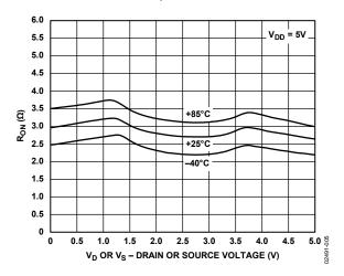
Figure 5. On Resistance as a Function of  $V_D$  ( $V_S$ ) for Different Temperatures  $V_{DD} = 5 V$
