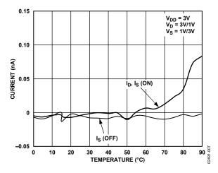
Figure 7. Leakage Currents as a Function of Temperature
