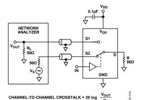
Figure 18. Channel-to-Channel Crosstalk
