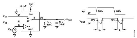
Figure 16. Break-Before-Make Time Delay,  $t_D$
