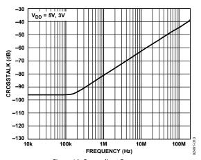
Figure 10. Crosstalk vs. Frequency
