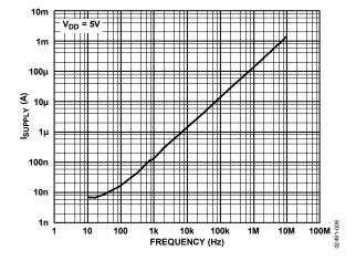
Figure 8. Supply Current vs. Input Switching Frequency
