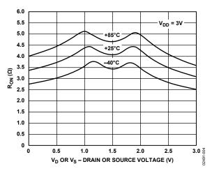
Figure 4. On Resistance as a Function of  $V_D$  ( $V_S$ ) for Different Temperatures  $V_{DD} = 3 V$
