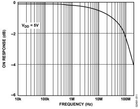
Figure 11. On Response vs. Frequency
